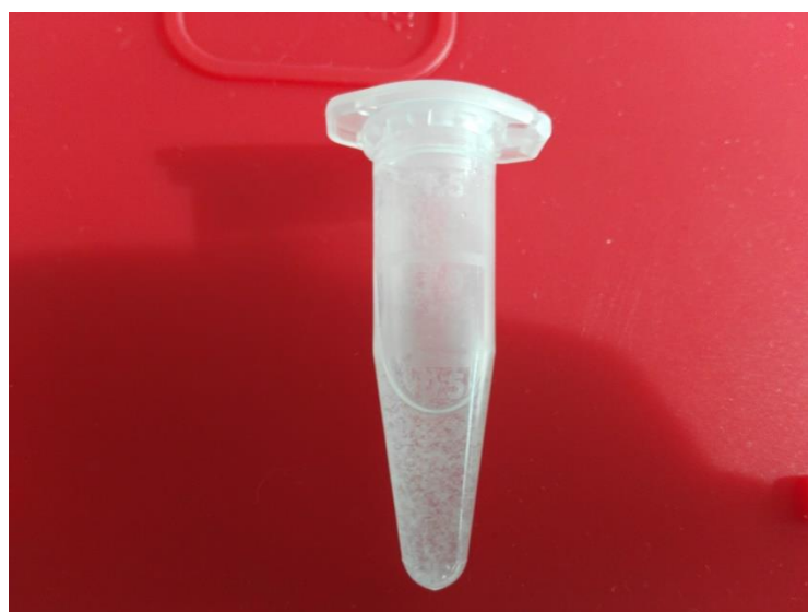
Figure 30. Solubility test of 0.5 mg FP in 1 mL of 25% DMSO, 50% ethanol, and 25% PBS.
