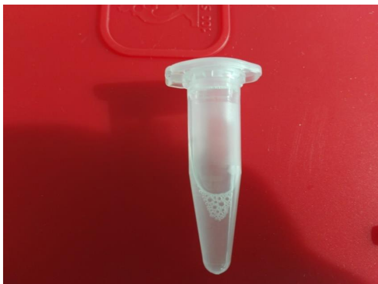
Figure 31. Solubility test of 0.5 mg FP in 1 mL of 1% DMSO and 0.1% Tween 80.
