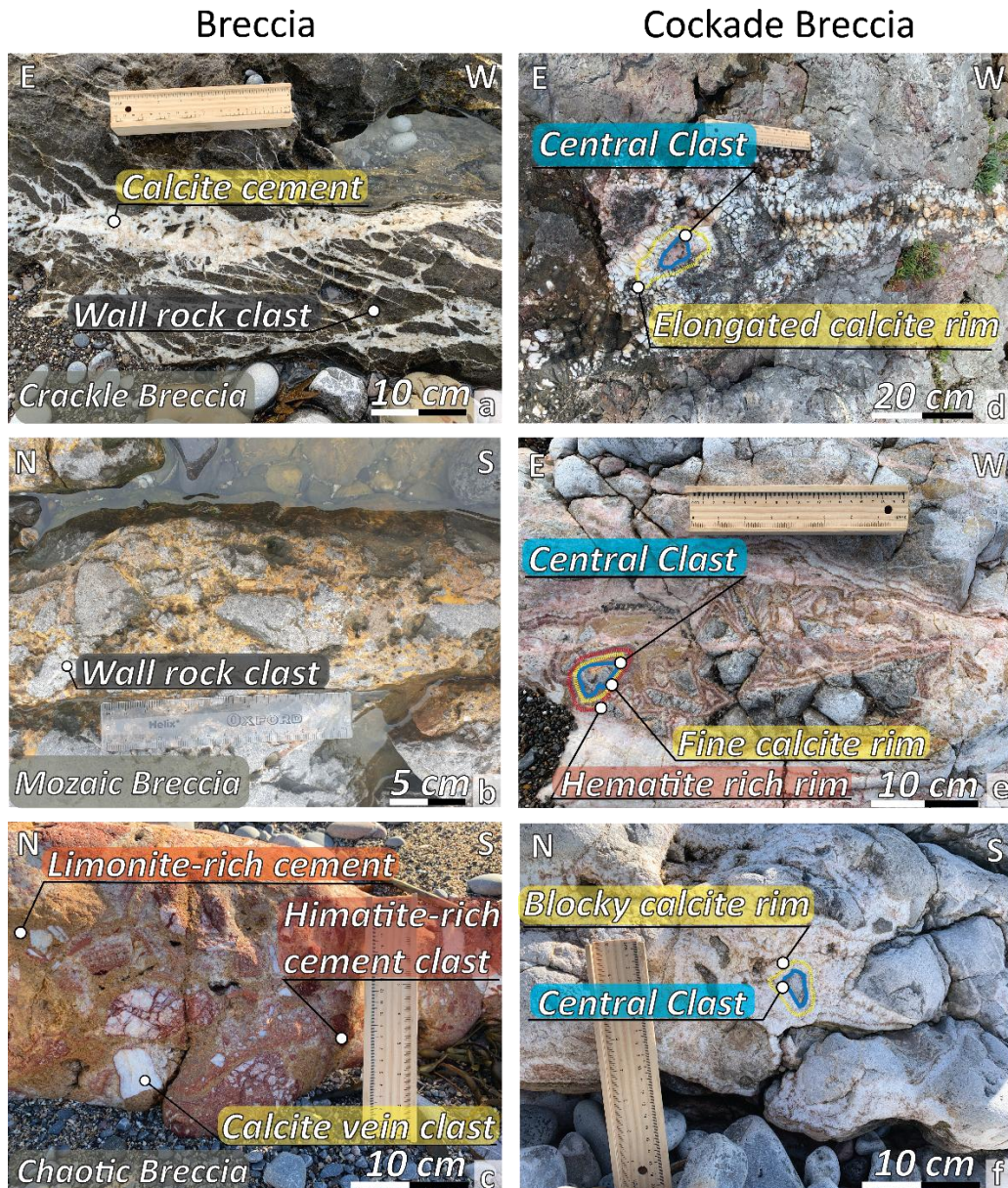
29: Breccia photos from the field and their UTM coordinates; a, b and c are the crackle, mosaic, and chaotic breccia respectively, (a- 419402 m E 5711059 m N; b- 417381 m E 5711370 m N; c- 419346 m E 5711056 m N); d- f) cockade texture having elongated, fine grain and hematite precipitate rims with wall rock originated limestone central clasts (d- 419245 m E 5711083 m N; e- 419410 m E 5711048 m N; f- 417098 m E 5711475 m N). (Datum: WSG84 UTM Zone)
