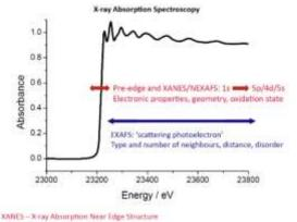
NEXAFS - Near Edge X-ray Absorption Fine Structure EXAFS - Extended X-ray Absorption Fine Structure
