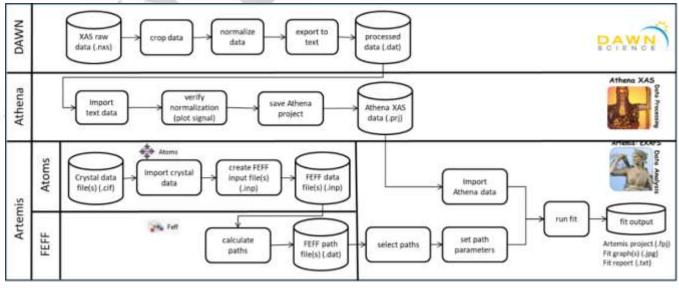
Figure 2 Schematic view of a XAS workflow. This workflow illustrates the processing and analysis of raw data using DAWN, Athena, Artemis, and two additional tools Atoms and FEFF. The workflow's complexity is evident in the number of inputs, outputs, and intermediate results, as well as the variety of file types involved.
