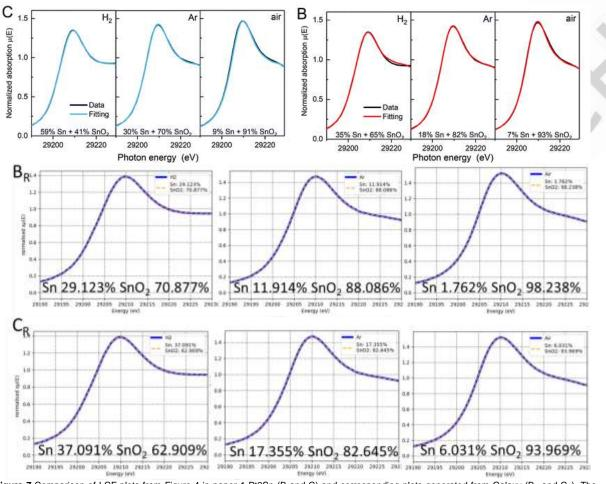
Figure 7 Comparison of LCF plots from Figure 4 in paper 1-Pt3Sn (B and C) and corresponding plots generated from Galaxy ( $B_R$  and  $C_R$ ). The main differences are because the Galaxy tools generate the LCF plots individually, and there is no option for combining and aligning plots. Additionally, the legends do not scale well. For this paper, we overlaid the percentages of the standards for better visibility.
