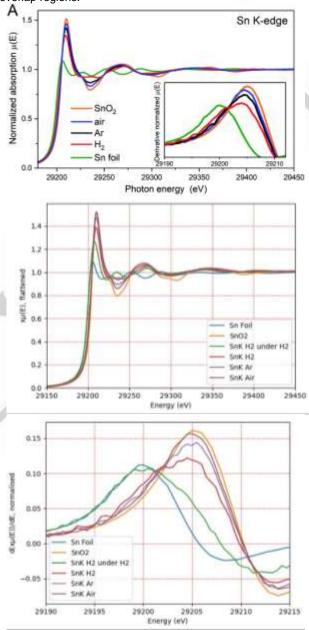
Figure 6 Comparison of XANES plots from Figure 4A in paper 1-Pt3Sn and equivalent plots generated from Galaxy. The top plot is the one included in the paper, the two plots under it are the ones produced in Galaxy. Note that Sn K edge of the H2 treated sample collected under H2 appears in the reproduction, to show how it was calibrated with respect to the other signals before using it in LCF
