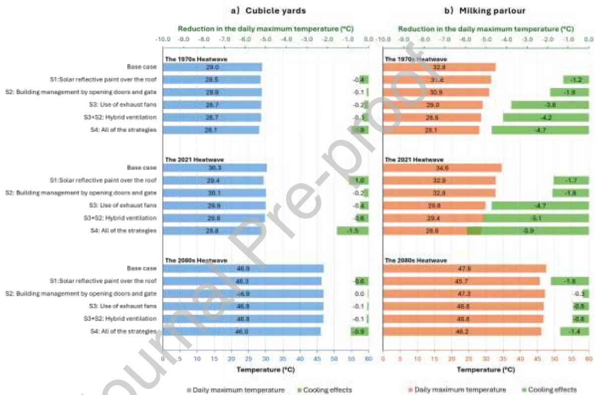
Figure 13. Comparison of mitigation strategies based on the daily maximum temperature ( \bar{T}_{daily}^{max} ) and their cooling effects, i.e., reduction in \bar{T}_{daily}^{max} in the cubicle yards throughout the day and in the milking parlour during the milking periods: 04:00-06:50 and 14:00-16:30.
