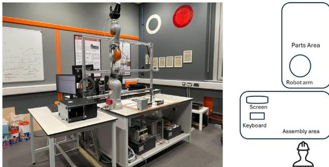
**Fig. 6.** The photo and layout diagram of the laboratory assembly line for Experiment 2.
