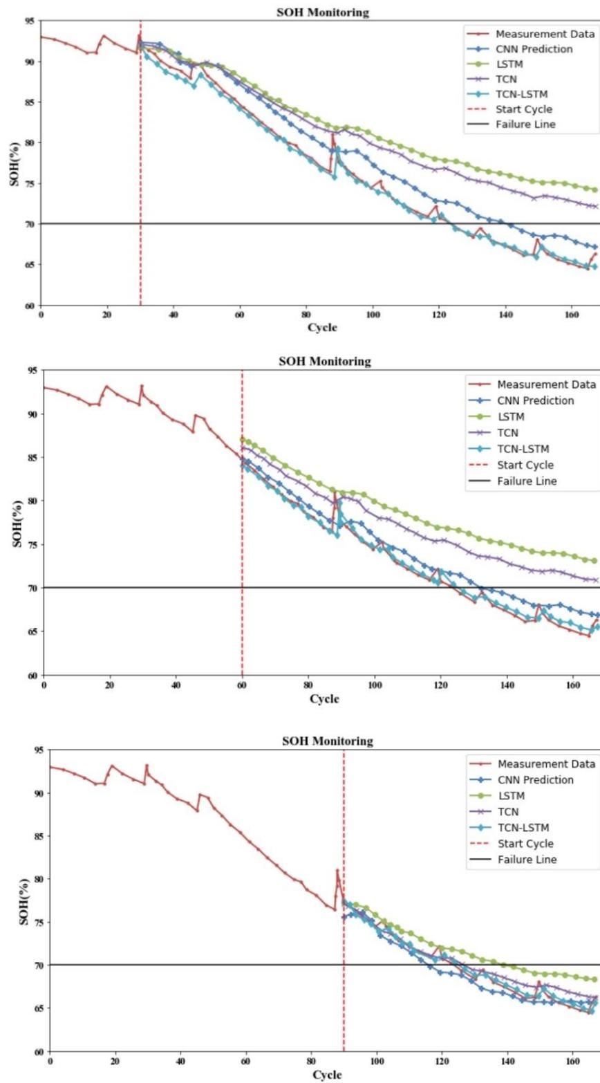
Figure 4. 10 The SOH monitoring of B0005 with 30th, 60th and 90th start cycle
