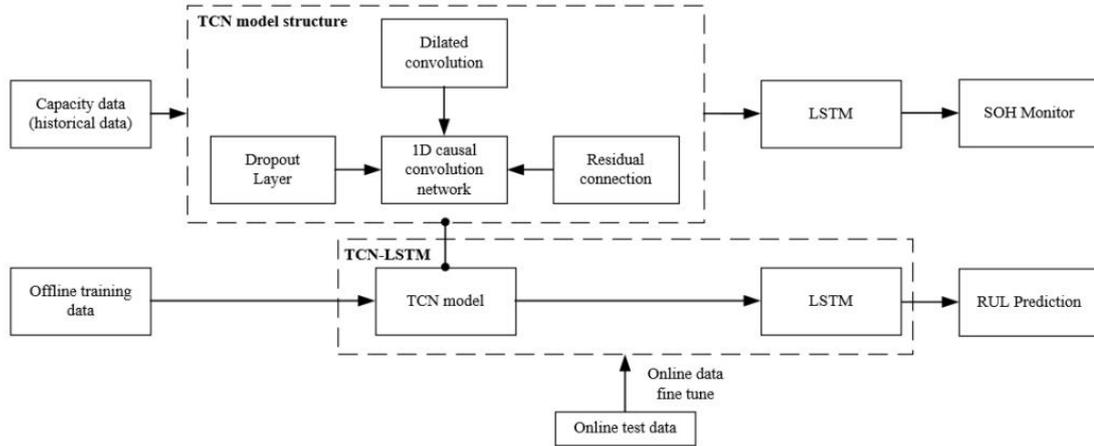
Figure 4. 5 The framework for battery health prognostics.
