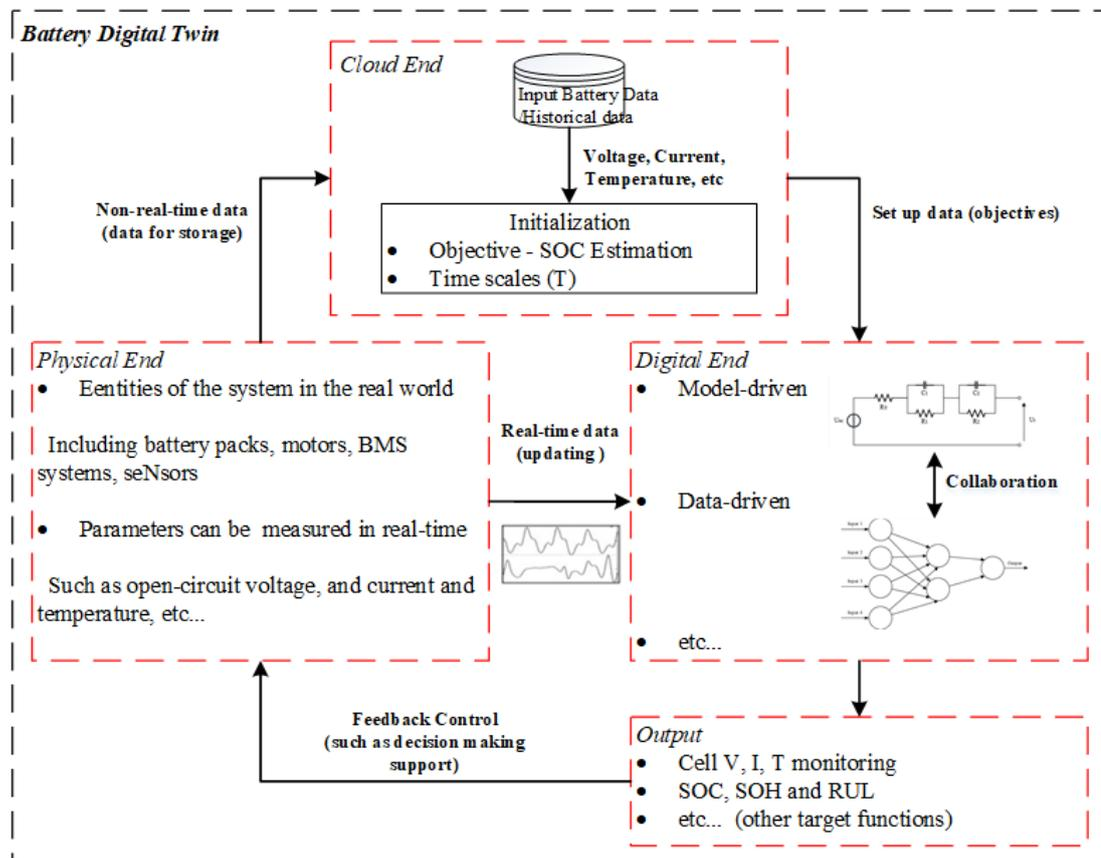
Figure 4.2 The battery digital twin framework for the proposed method.
