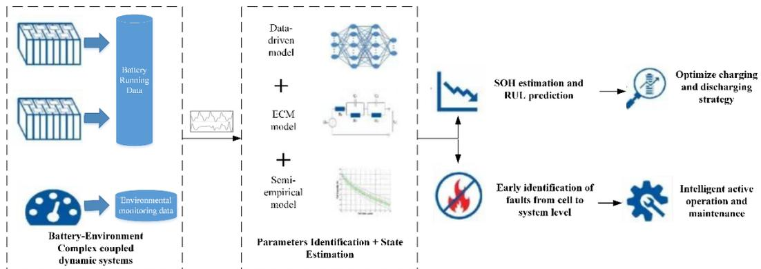
Figure 4.1 State estimation for the battery-environment coupled systems.
