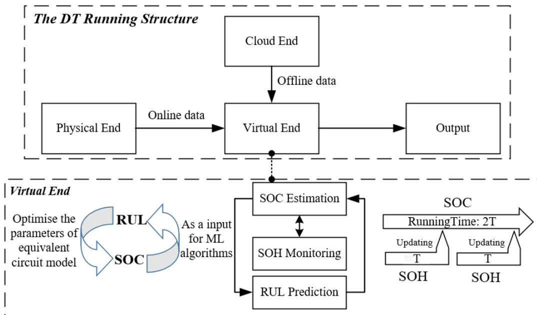
Figure 4. 7 Schematic diagram of DT running.
