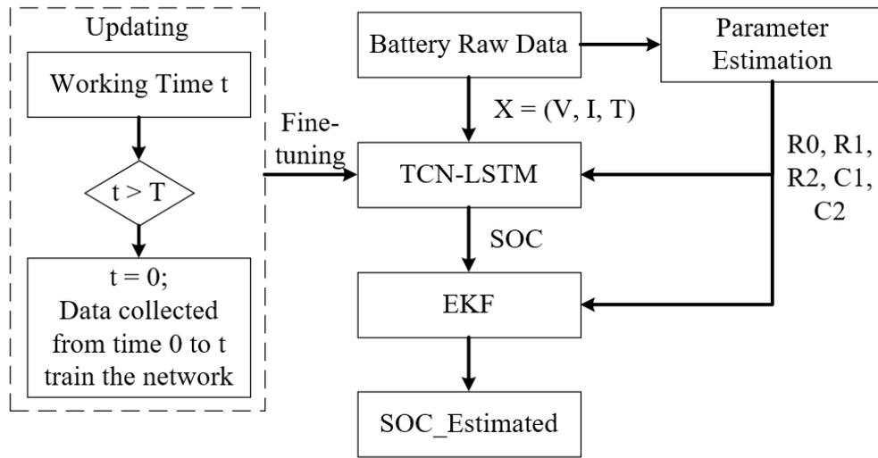
Figure 4.4 Flowchart of the SOC estimation in Digital End.
