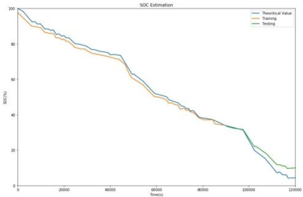
Figure 4. 9 The SOC estimation by TCN-LSTM
