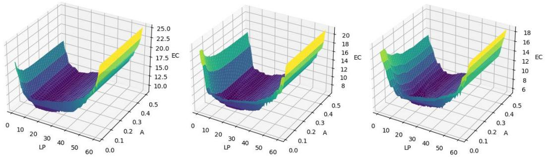
Figure 6. 1 The expected cost per unit time in terms of the preventive maintenance threshold  $L_p$  and the availability  $A$  with different period  $T$  ( $T=100, 200, 300$ )
