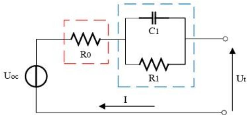
Figure 5.1 The first-order ECM for a lithium-ion cell.
