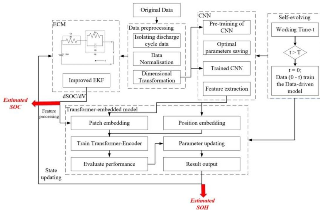
Figure 5. 2 The Transformer-CNN model within the HSE-DT method
