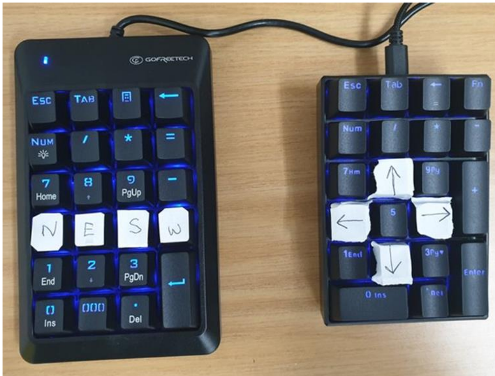
Figure 7 shows the USB NUM pads on which participants responded when taking part in Experiment 2. The left-most NUM pad has four keys, each one marked with one of the following letters: N, E, S and W. This NUM pad is the ‘verbal’ response pad. The right-most NUM pad is marked with four directional arrows representing the cardinal directions of North, East, South and West.
