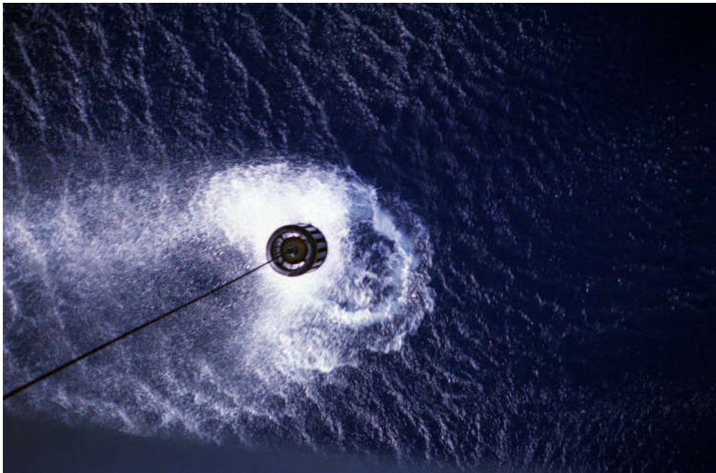
Figure 2.11: An AQS-13 dipping sonar being lowered from an SH-3D Sea King helicopter from Helicopter Anti-submarine Squadron 2 (HS-2). Courtesy of the U.S. Department of Defense [103]
