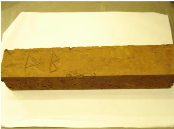
Figure 5.9 Photograph of a cast block after 6 days curing produced from the addition of cement to the sludge from Horden. The block is 250mm long and 50mm square.
