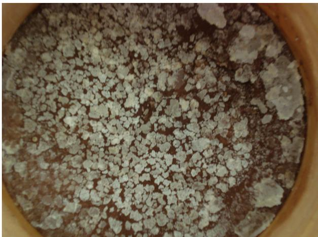
Figure 8.4 Calcite crust on the top of column 1
