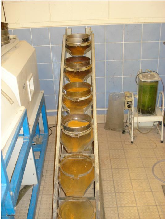
Figure 5.10 Photograph of the vibrating sieve used to separate the pellets into the desired size fractions.
