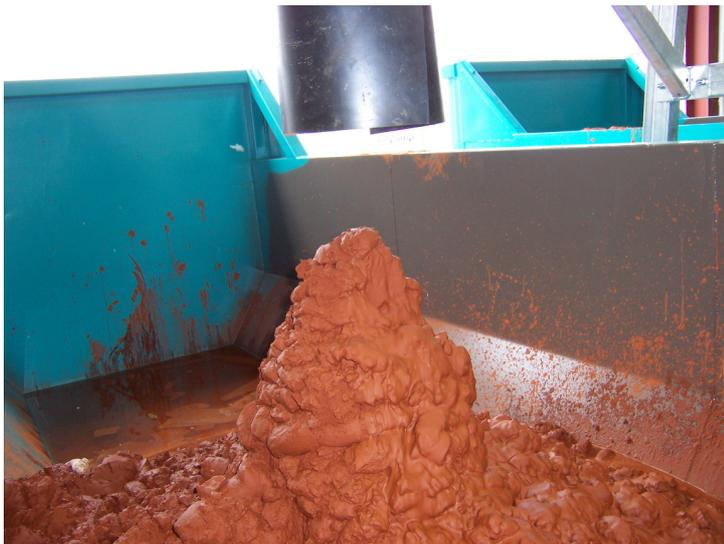
Figure 5.1 Photograph showing the treated sludge form Horden minewater treatment plant as it is discharged from the centrifuge at the treatment plant.
