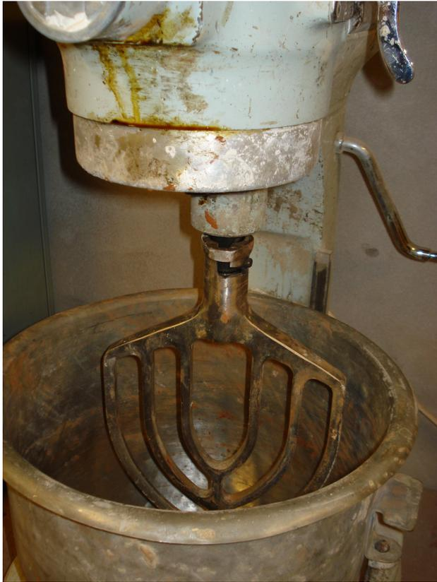
Figure 5.8 Photograph of the dough type mixer used for the mixing of cement and the sludge from Horden minewater treatment plant
