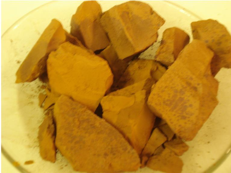
Figure 5.4 Photograph of the solids from the Dawdon minewater treatment plant
