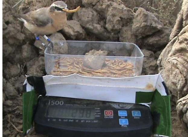
Fig. 2.3. Second-year (young) male wheatear ( O. o. leucorhoa ) with colour rings (right leg: dark blue/metal, left leg: white/white/dark blue) using remote weighing set up in PNOD. The rocks and cattle dung positioned around the balance and bowl of dried mealworms are to reduce the effect of wind on the balance readings. Cardboard is attached to the front of the balance to shade the LCD from the sun, increasing its visibility. The balance reading is 29.8 g.
