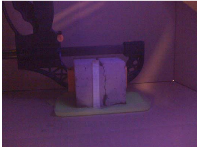
Figure 13: Image of natural crack experimental arrangement under UV lighting
