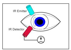
Figure 2.16 Illustration of the infrared oculography technique (http://www.liv.ac.uk /~pcknox/teaching/Eymovs/params.htm).
