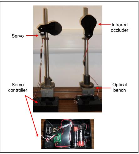
Figure 3.15 Semi-automated occluder unit.
