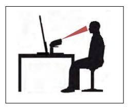
Figure 7.6 Optimum setup for the Tobii X120 eye tracker (Tobii Studio<sup>™</sup> 2.2 User Manual 2010).
