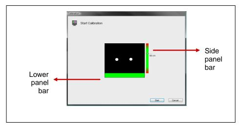
**Figure 4.4** Initial set up prior to calibration to determine the subject's distance from the eye tracker. The calibration window will automatically give the distance measurement from the eye tracker to the subject's eyes, as shown at the side panel bar. Lower panel bar represents the strength of the infrared transmission.
