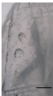
Figure 4.9 Representative light photomicrograph of SGMN array containing \beta -galactosidase following insertion into human skin.
