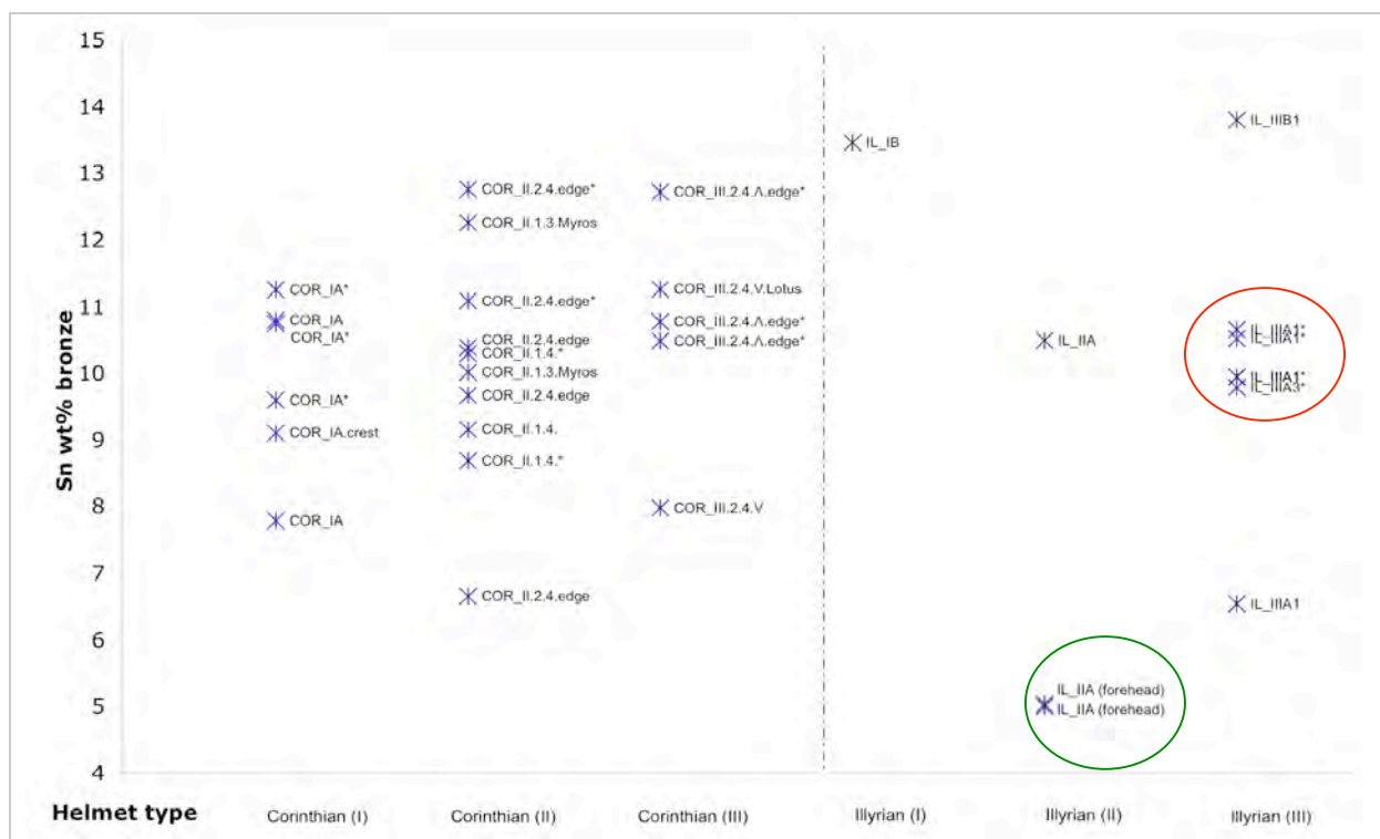
Figure 5.24: Sn wt% concentration of samples plotted against chronological phase of helmet type. Left: Corinthian type helmets exhibiting a slight trend for increasing tin content at the Late Phase III. Right: Illyrian type helmets showing clustering of Sn composition based on provenience (green, Aghia Paraskevi) or stylistic subgroup (red).
