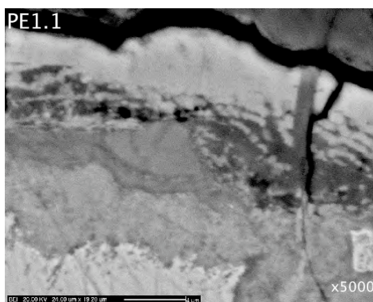
Figure 6.15: BSE and SE images showing the nature of the grey/silver patina in PE1.1 in cross-section. SEM-EDX map of OK \alpha , SnLa and CuKa shows spatial distribution of elements in patina. The patina appears orange/yellow in BSE but it is richer in Sn than in Cu. The key notes X-ray counts of SnLa.
