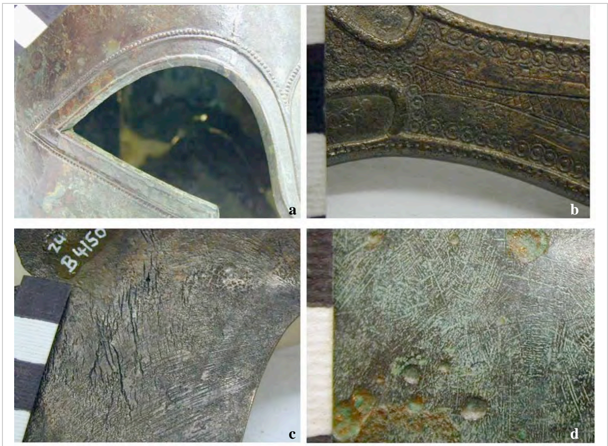
Figure 5.8: Examples of cast features on helmets. (a) Cast noseguard and decoration (OL_B10518). (b) Cast and punched decoration on noseguard (OL68). (c) Casting shrinkage and crude filing marks at the back of noseguard (OL68). (d) Dendritic microstructure on the crown of OL80 (Myros group) emphasised by corrosion.
