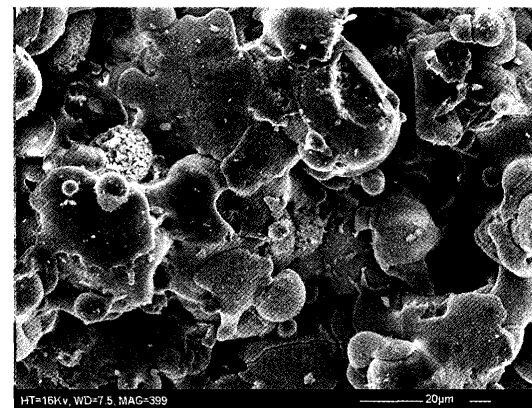
Fig. 2 SEM images of the \beta TCP coated screw. (A) Low magnification. (B) High magnification.
