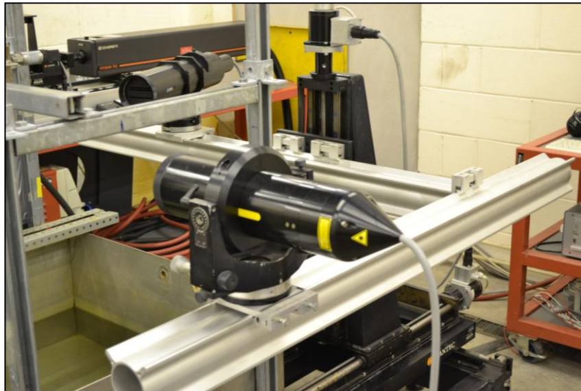
Figure 3.4.1 The computer-controlled traverse with sending and receiving optics mounted.
