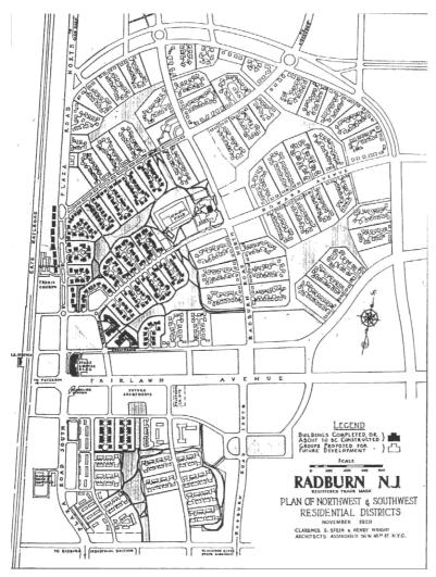
Figure 2- 2: The plan of Radburn, New Jersey - neighbourhood units with residential cul-de-sacs and segregated transport modes, clustered around a centrally located high school, Source: http://www.cmhpf.org/surveymecklenburgpaper.htm
