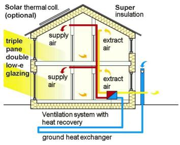
Figure 2-7: Diagram explaining the principles of Passivhaus, Source: (Mead and Brylewski 2011)
