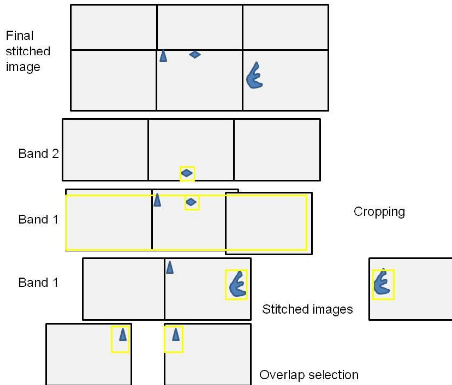
Figure 2.21 Stitching of high resolution images. Figure illustrates how overlaps of images are selected to generate a merged image. This is performed in bands to allow stitching in 2 dimensions. Once a band is finished, cropping allows for better overlap to stitch individual bands together.
