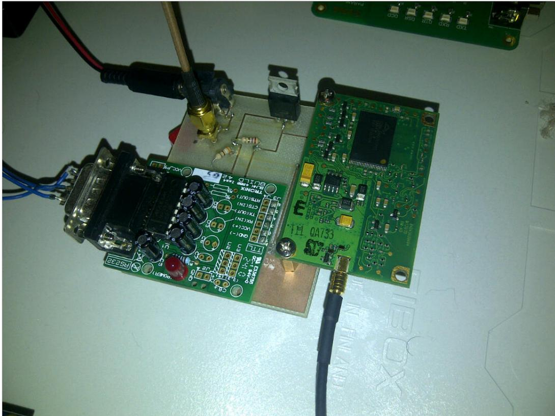
Figure 7.17: GPS Timestamping module PCB including the M12M Timing Receiver and the RS-232 interface to to the FPGA
