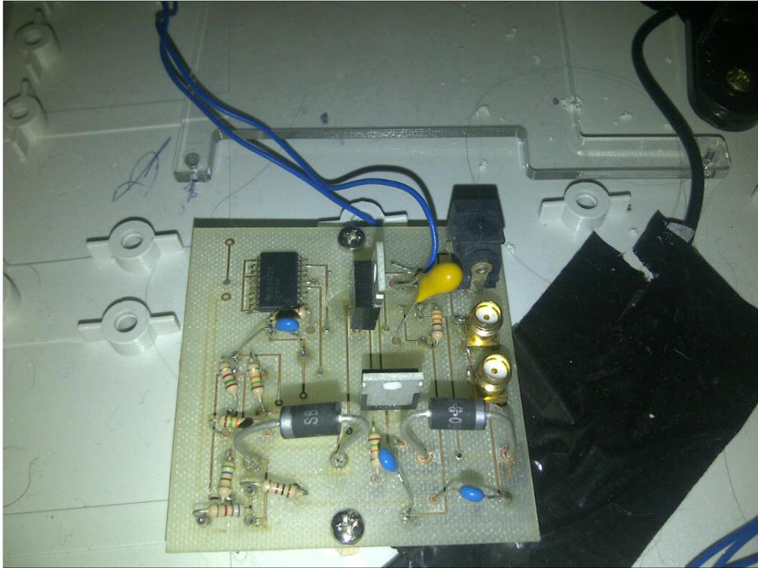
Figure 7.19: The OPA564 and biasing circuitry PCB board including 24V supply, input/output sma connectors and wires leading to “on/off” switch for external mounting
