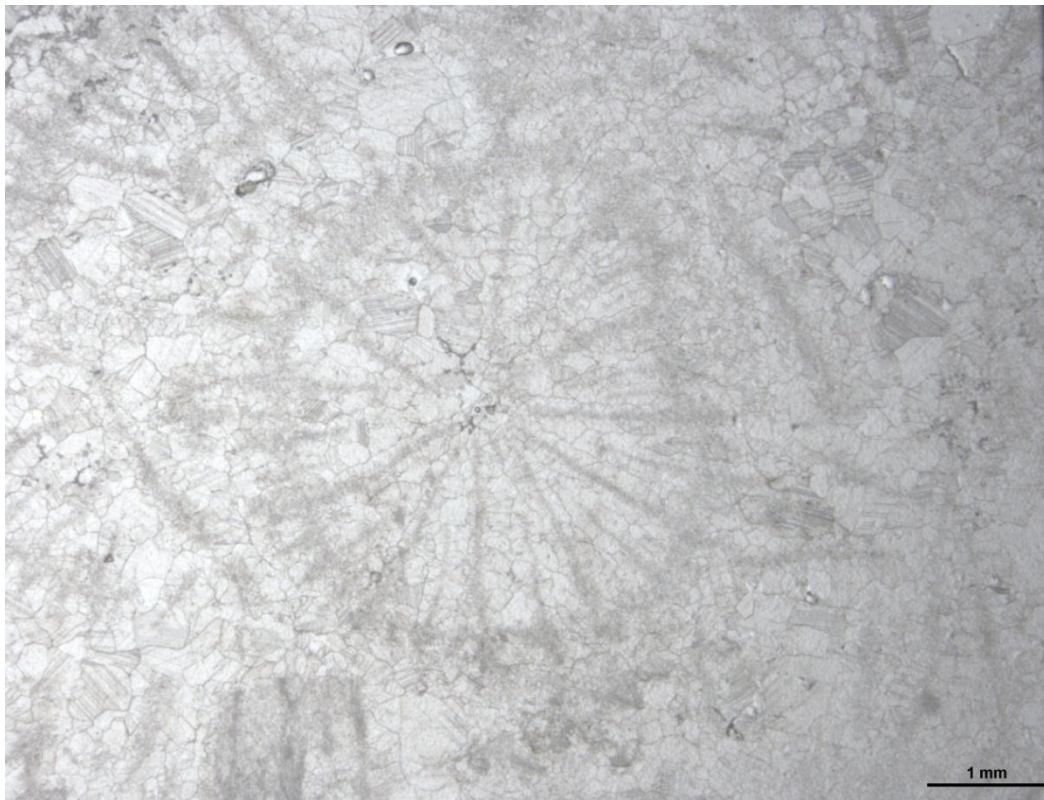
Figure 5.6: Photomicrograph of aragonitic coral altered by calcite spar in which the relict of original coral is retained. Un-stained thin-section from Core of Aj Dagh Anticline (sample number CA.19).
