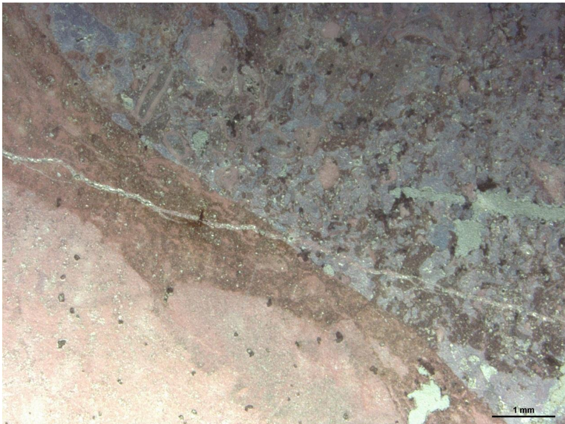
Figure 5.14: Photomicrograph of non-ferroan calcite spar filled fracture cuts both non-ferroan and ferroan calcite spar. Stained thin-section from Zinana area (sample number Z.30).
