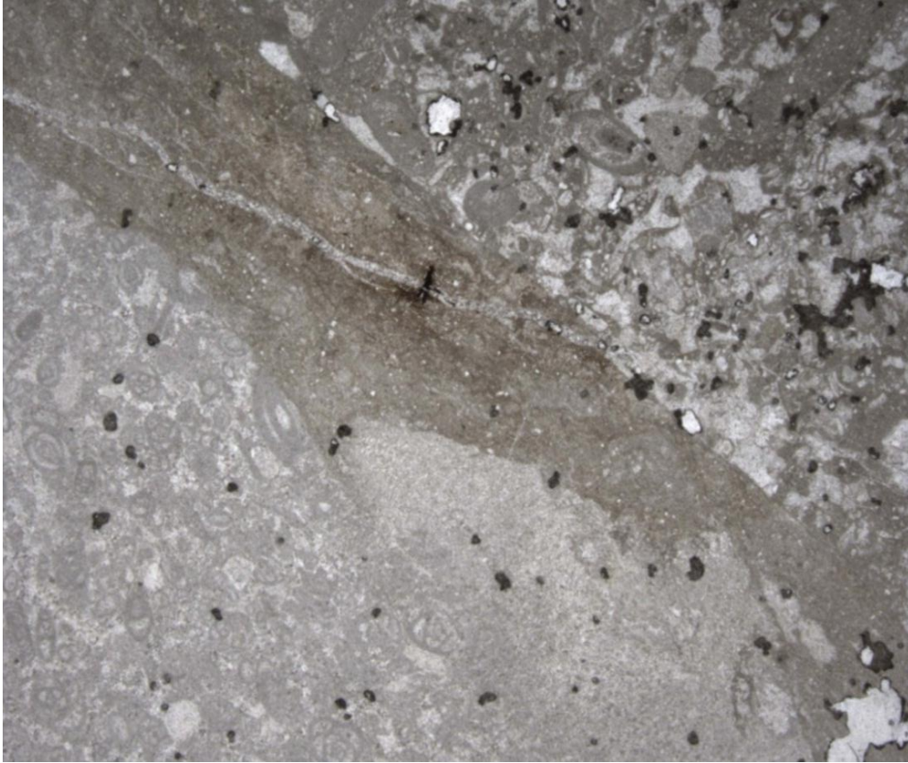
Figure 5.12: Early cement associated with hardground with criteria of grain truncation (1), micro-boring (2) and planar surface(3). Un-stained thin-section from Zinana locality. Scale 1cm=1mm.
