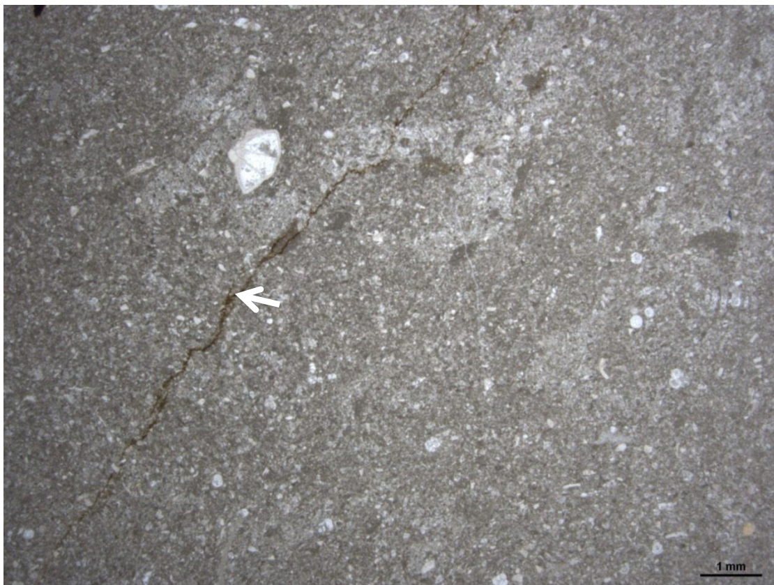
Figure 4.41: Photomicrograph of PK-2 with clay seams (arrowed). Unstained thin-section at Bellula Gorge locality (sample BL.32).
