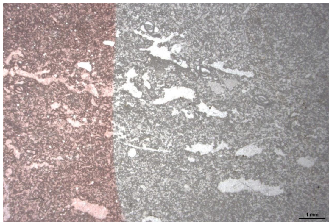
Figure 4.26: Photomicrograph of fenestral pores filled with non-ferroan calcite cement. The thin-section is half stained from the core of Aj Dagħ Anticline (sample CA.16).
