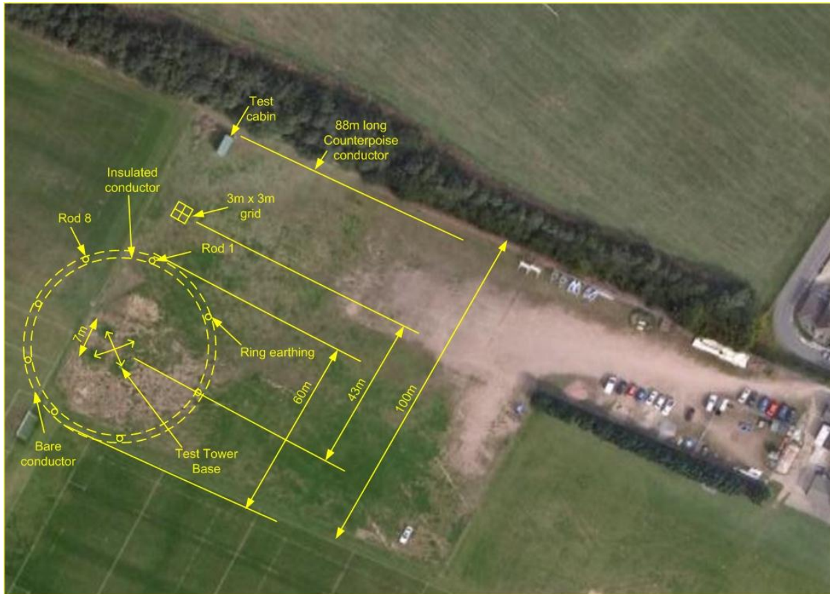
Figure 4.1 Plan view of University test site at Llanrumney showing outline of installed test electrodes
