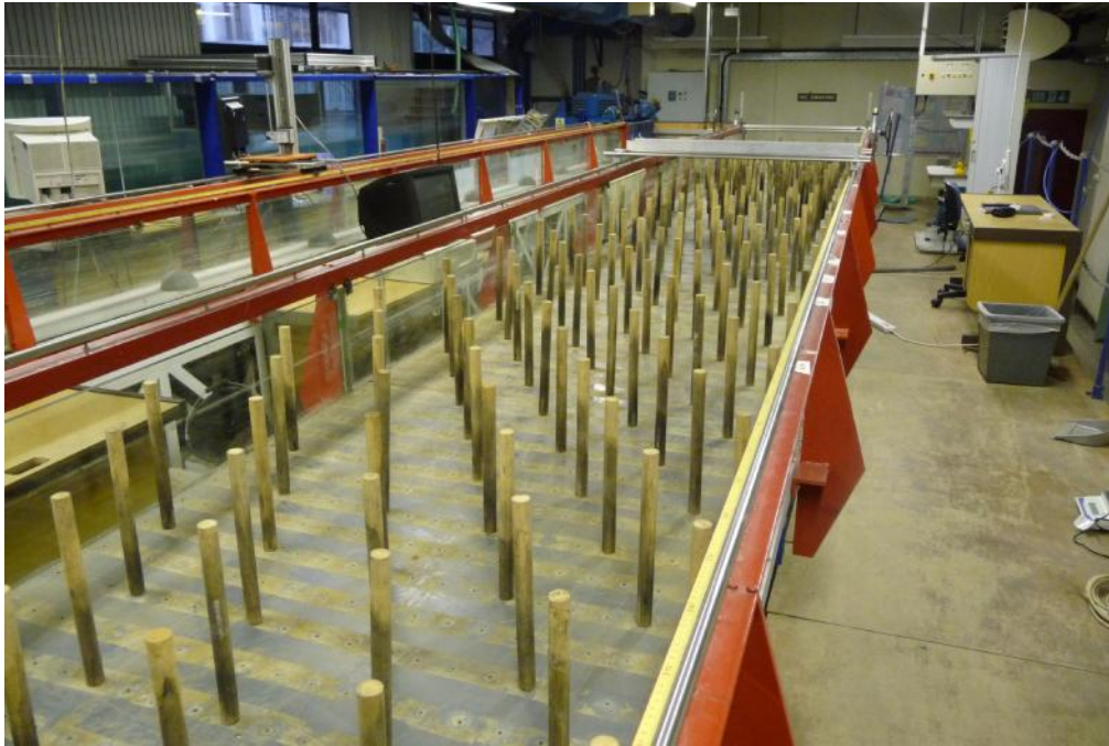
Figure 3.5 (b) Rods in staggered arrangement for test 0.97S
