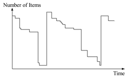
Figure 2: Example of possible information gathered by scale based monitoring system
