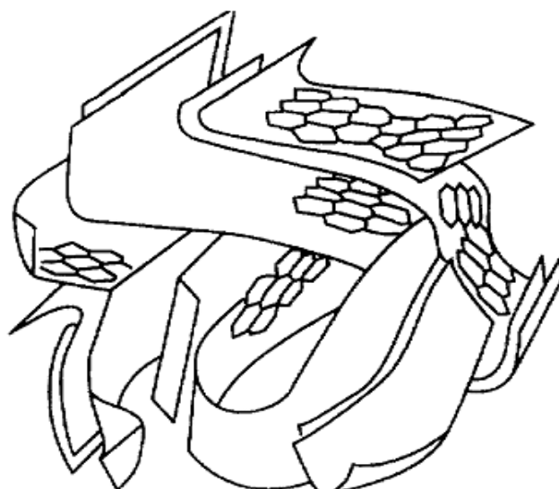
Figure 4.1 Schematic of the structure of activated carbon showing planes of graphitic structures overlapping and in-between plane space corresponding to micro porous features 6 .
