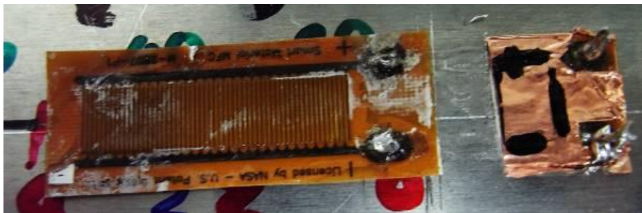
Figure 2-6. Original M2807-P1 transducer and the final cut down version
