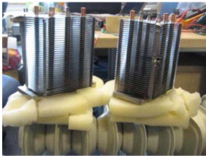
Figure 4-6. TEG energy harvesting device for a automatic valve controller (Lu and Yang 2010)
