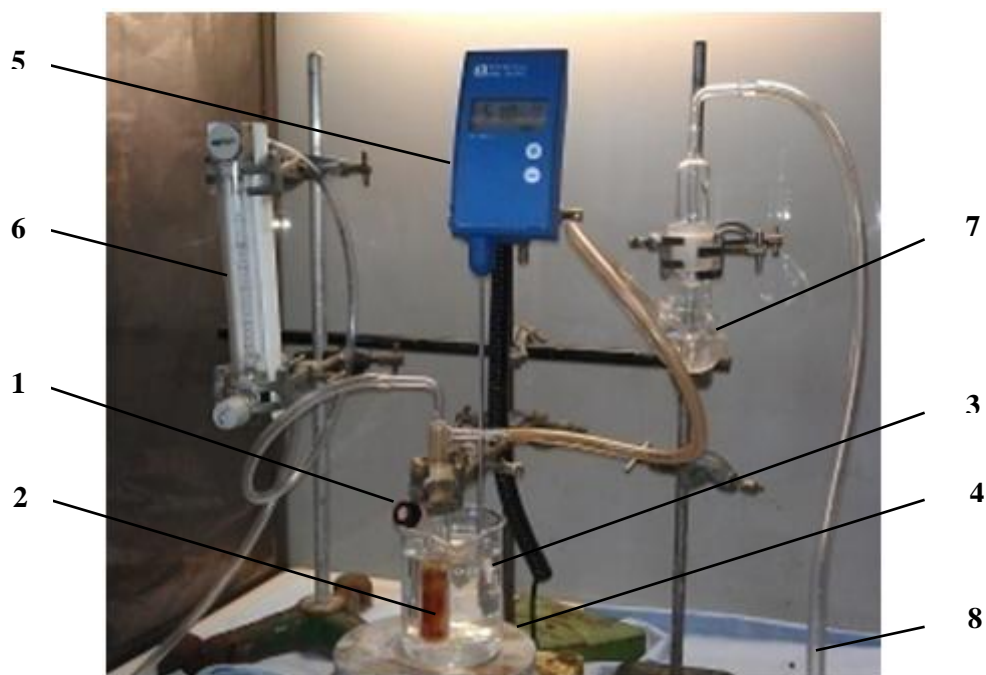
Figure 2.12. NOA setup for plasma nitrite and/or RSNO measurement. 200 \mu\text{l} sample (+ few drops of Antifoam TM ) is injected through the rubber septum (1) into a specially constructed purge vessel with 5 ml tri-iodide reagent (2). The temperature of the reagent is maintained at 50 °C by a beaker of water (3) kept on a hot plate (4) linked to IKATRON® ETS-D4 fuzzy (5). Released NO is carried in an inert N 2 gas stream controlled by a flowmeter (6; flow: 200 cm 2 /min) to a round-bottom flask with 1 M NaOH (7). NaOH protects NOA from damage by hot acid vapour and ensures that N-oxide contaminants are not converted to NO (no false positives). Neutralized NO vapour is directed to NO analyser (8).
