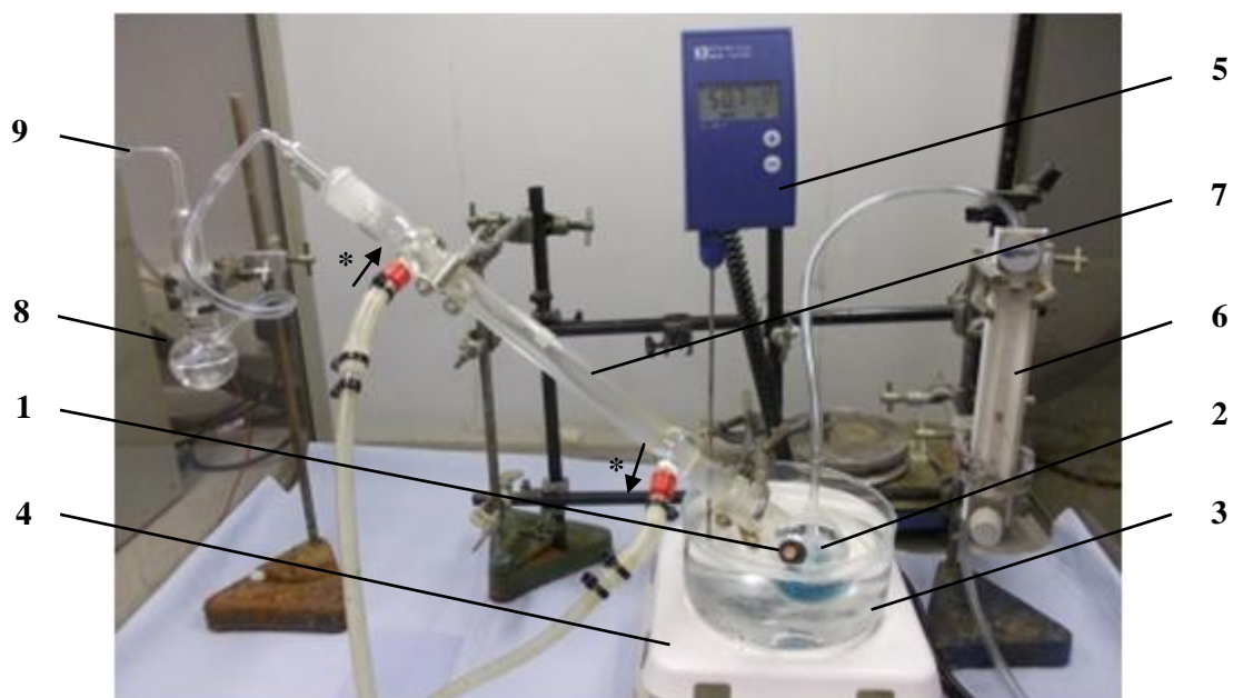
Figure 2.15. NOA setup for plasma nitrate measurement. 20 \mu\text{l} sample is injected through the rubber septum (1) into a 2-neck round bottom flask with 30 ml vanadium chloride reagent (2). The temperature of the reagent is maintained at 85 ^{\circ}\text{C} by a beaker of water (3) kept on a hot plate (4) linked to IKATRON® ETS-D4 fuzzy (5). Released NO is carried in an inert N_2 gas stream controlled by a flowmeter (6; flow: 200 \text{cm}^2/\text{min} ) and directed through a condenser (7) to a round-bottom flask with 1 M NaOH (8). The water flow in the condenser was unconventional (*). The condenser and NaOH protects NOA from damage by very hot acid vapour. Neutralized NO vapour is directed to NOA analyser (9).
