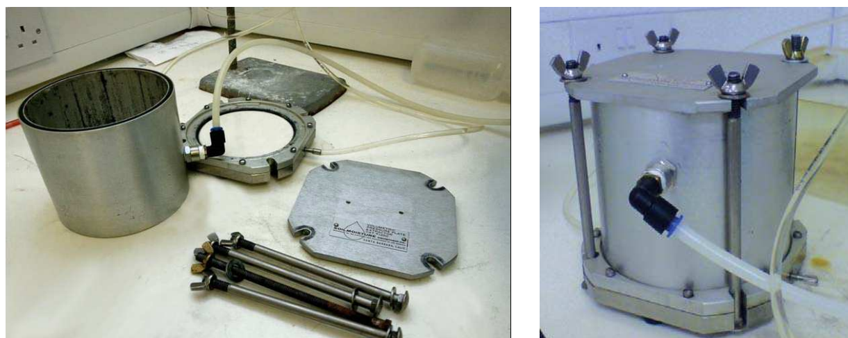
Fig. 3.11 2-bar volumetric pressure plate
