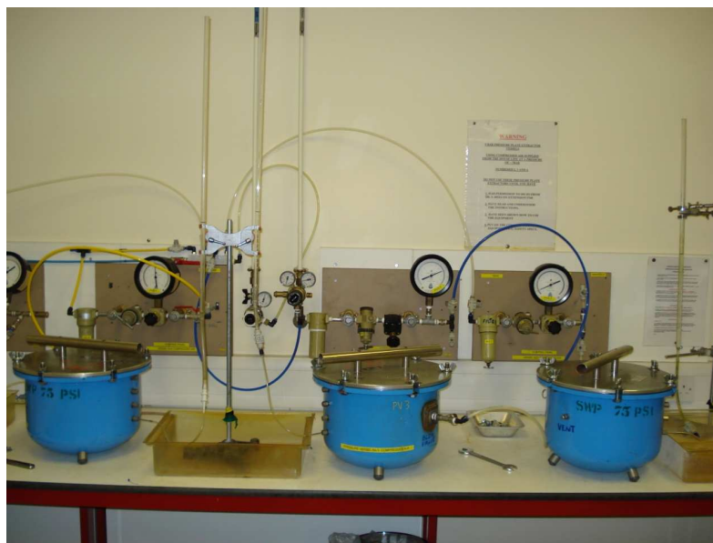
Fig. 3.9 5-bar pressure plate extractor
