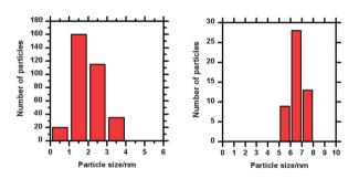
**Fig. 4** Au nanoparticle size distributions for Fig. 3b and 5b (before and after heating to 573 K for 1 minute). Heating has resulted in the sintering of small gold nanoparticles and the formation of a smaller number of larger particles.
