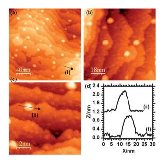
Fig. 5 STM images of the  $\gamma\text{-Fe}_2O_3$  (2  $\times$  2) surface after deposition of Au and subsequent heating to 573 K for 1 minute.
