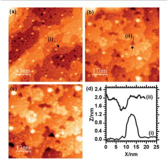
**Fig. 6** STM images taken after the deposition of Pd onto the  $Au/\gamma$ -Fe<sub>2</sub>O<sub>3</sub> surface. Particles with widths of  $\sim$ 10 nm can be assigned to Au, smaller particles are due to the Pd.
