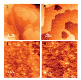
**Fig. 1** STM images of the clean  $\gamma$ -Fe<sub>2</sub>O<sub>3</sub> (2 × 2) surface prepared by sputtering and annealing in vacuum for 20 minutes at 873 K.
