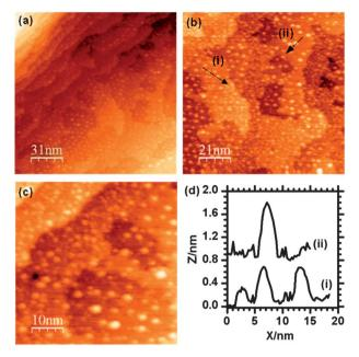
**Fig. 3** STM images of the  $\gamma$ -Fe<sub>2</sub>O<sub>3</sub> (2  $\times$  2) surface after deposition of Au. The majority of particles are in the range of 1 to 3 nm in diameter with larger particles being up to 4 nm. The particle size distribution is summarised in Fig. 4.
