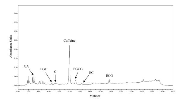
Figure 3.33. HPLC profile of black tea BP-5 at 210 nm.
