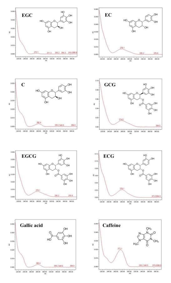
Figure 3.30. The UV spectra of catechins, gallic acid and caffeine between 200 – 400 nm.
