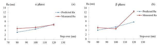
**Figure 10.** Experimental and predicted results for the arithmetic roughness, Ra, for (a) the  $\alpha$  phase and (b) the  $\beta$  phase.
