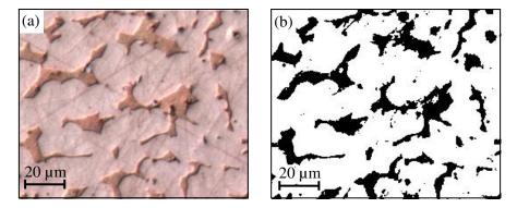
**Figure 3.** Material microstructure mapping procedure, (a) optical micrograph of the  $CuZn_{39}Pb_3$  brass alloy sample, (b) processed binary picture from the optical micrograph.
