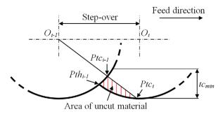
**Figure 2.** Surface generation in the feed direction during AFM probe-based machining.
