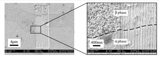
**Figure 8.** Example of a machined pocket with a step-over of 100 nm. The dashed line represents the boundary between the  $\alpha$  and  $\beta$  phases.
