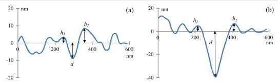
**Figure 6.** Examples of cross sections of a machined groove in the  $\alpha$  phase at (a) the ploughing to cutting transition point and (b) under pure cutting mechanism.
