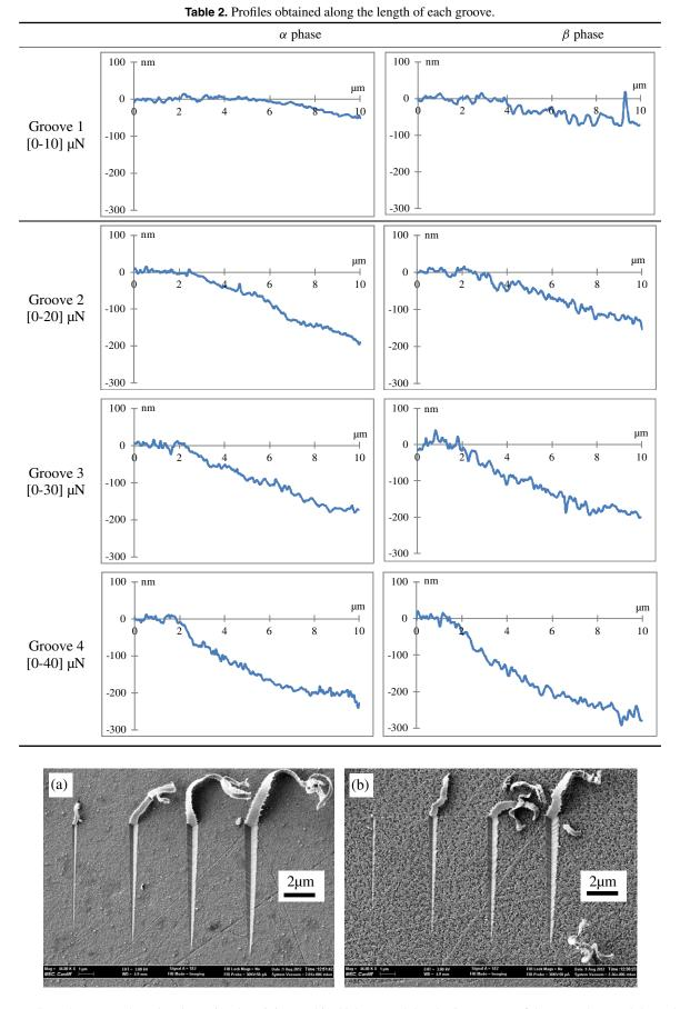
Figure 5. Scratch tests conducted to determine the minimum chip thickness and the elastic recovery of the (a)  $\alpha$  phase and (b)  $\beta$  phase.
