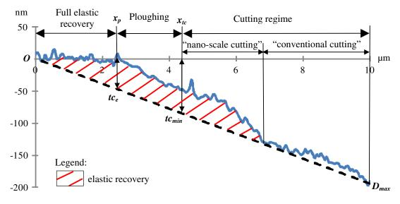
Figure 7. Illustration of the procedure used to determine the minimum chip thickness and the elastic recovery values for a particular scratched groove.
