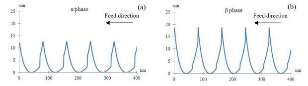
**Figure 9.** Predicted surface profile along the cross section of a series of parallel grooves with a step-over value of 80 nm for (a) the  $\alpha$  phase and (b) the  $\beta$  phase.
