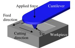
**Figure 1.** Schematic representation of the AFM probe-based mechanical machining process when producing a pocket.
