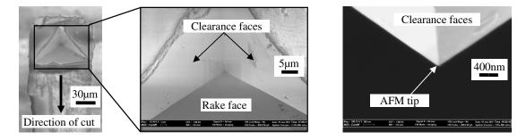
Figure 4. Tip of the DNISP AFM probe.
