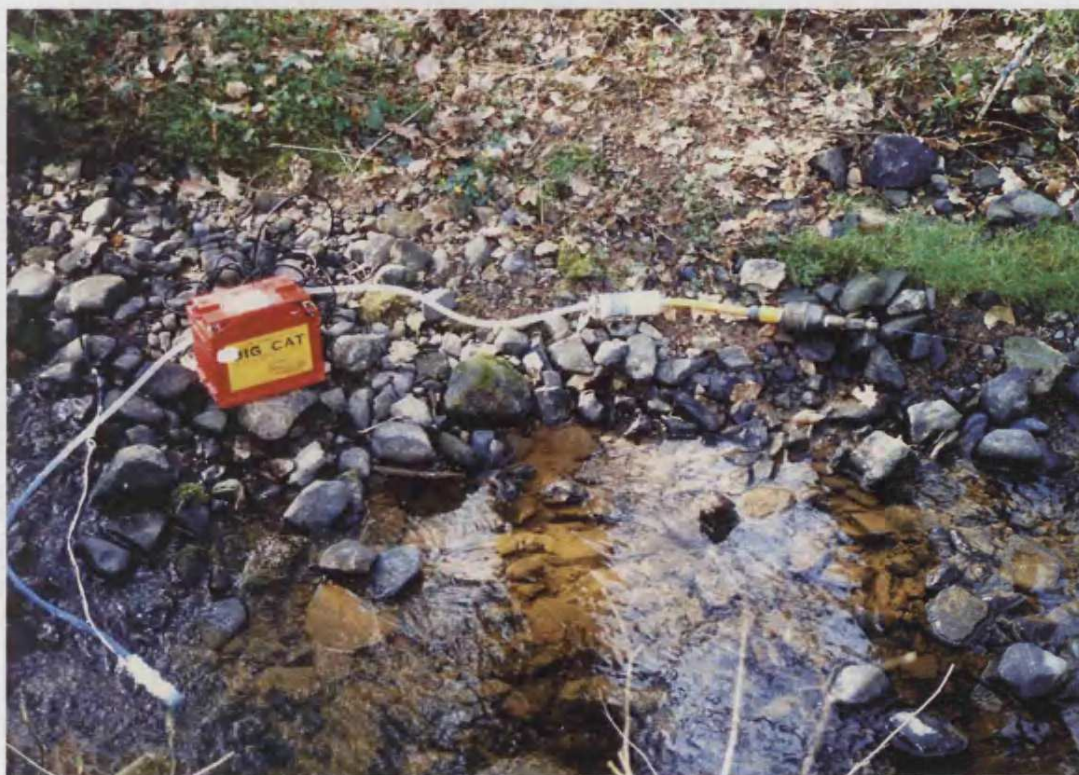
Figure 5.5: A photograph showing the battery-powered rig, sampling water from the pump submerged in the stream, through the filter capsule and through the water meter before releasing the filtered water back into the stream.
