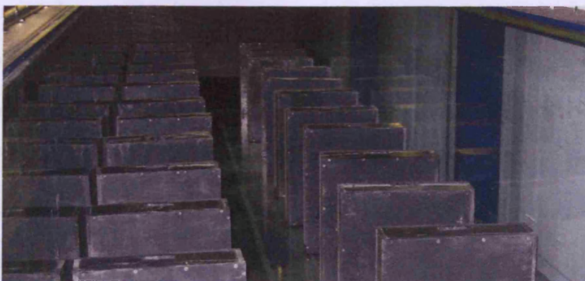
Figure 6.11 View of PVC Blocks used to construct floodplain physical model
