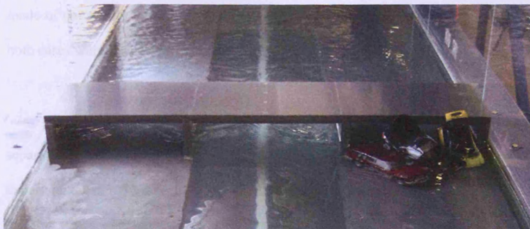
Figure 6.15 Physical model of floodplain with model vehicle blockages for three different designs of scaled model bridge
