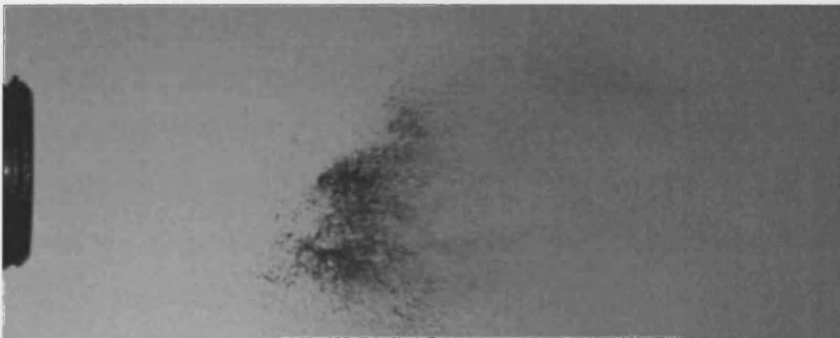
Figure 6.20g: Pulsed Flow Breakup, z=20\text{mm} , Frame 7
