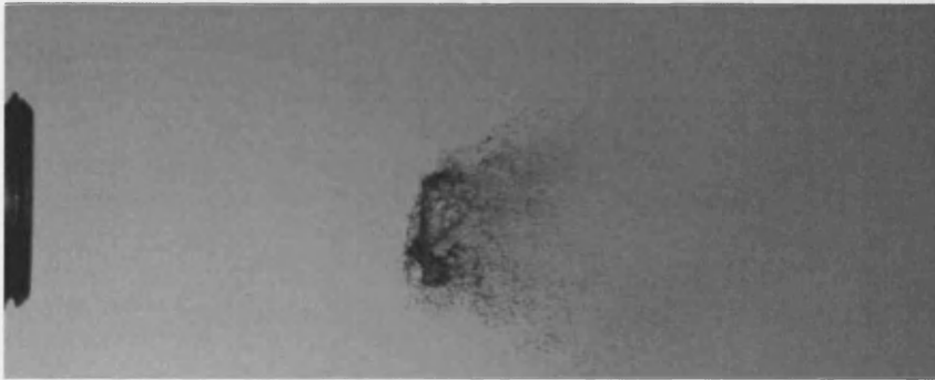
Figure 6.21f: Pulsed Flow Breakup, z=30\text{mm} , Frame 6
