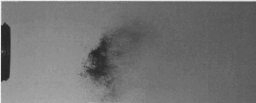
Figure 6.20f: Pulsed Flow Breakup, z=20\text{mm} , Frame 6
