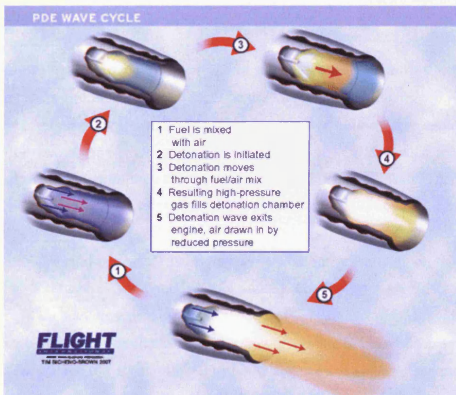
Figure 1.5: PDE Engine Cycle [14]
