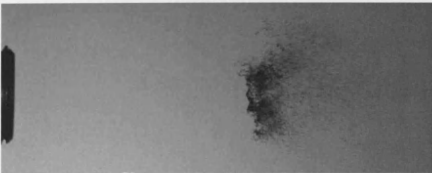
Figure 6.22g: Pulsed Flow Breakup, z=40\text{mm} , Frame 7
