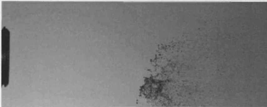
Figure 6.21j: Pulsed Flow Breakup, z=30\text{mm} , Frame 10
