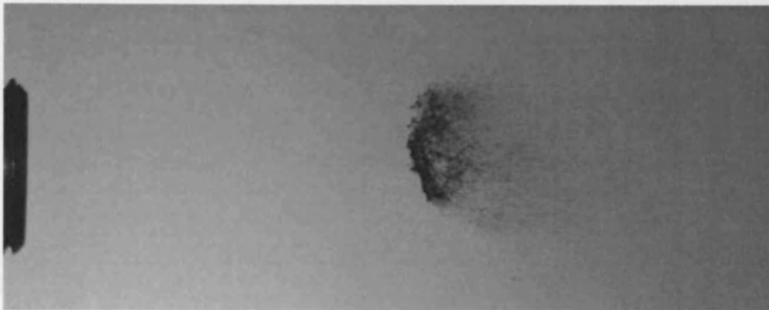
Figure 6.22e: Pulsed Flow Breakup, z=40\text{mm} , Frame 5
