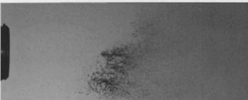
Figure 6.20h: Pulsed Flow Breakup, z=20\text{mm} , Frame 8
