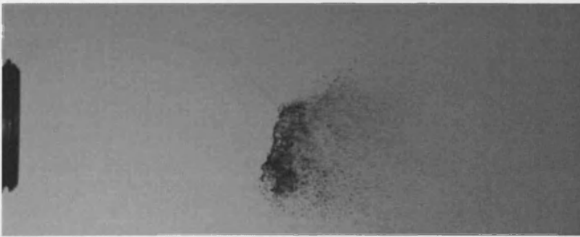
Figure 6.21g: Pulsed Flow Breakup, z=30\text{mm} , Frame 7
