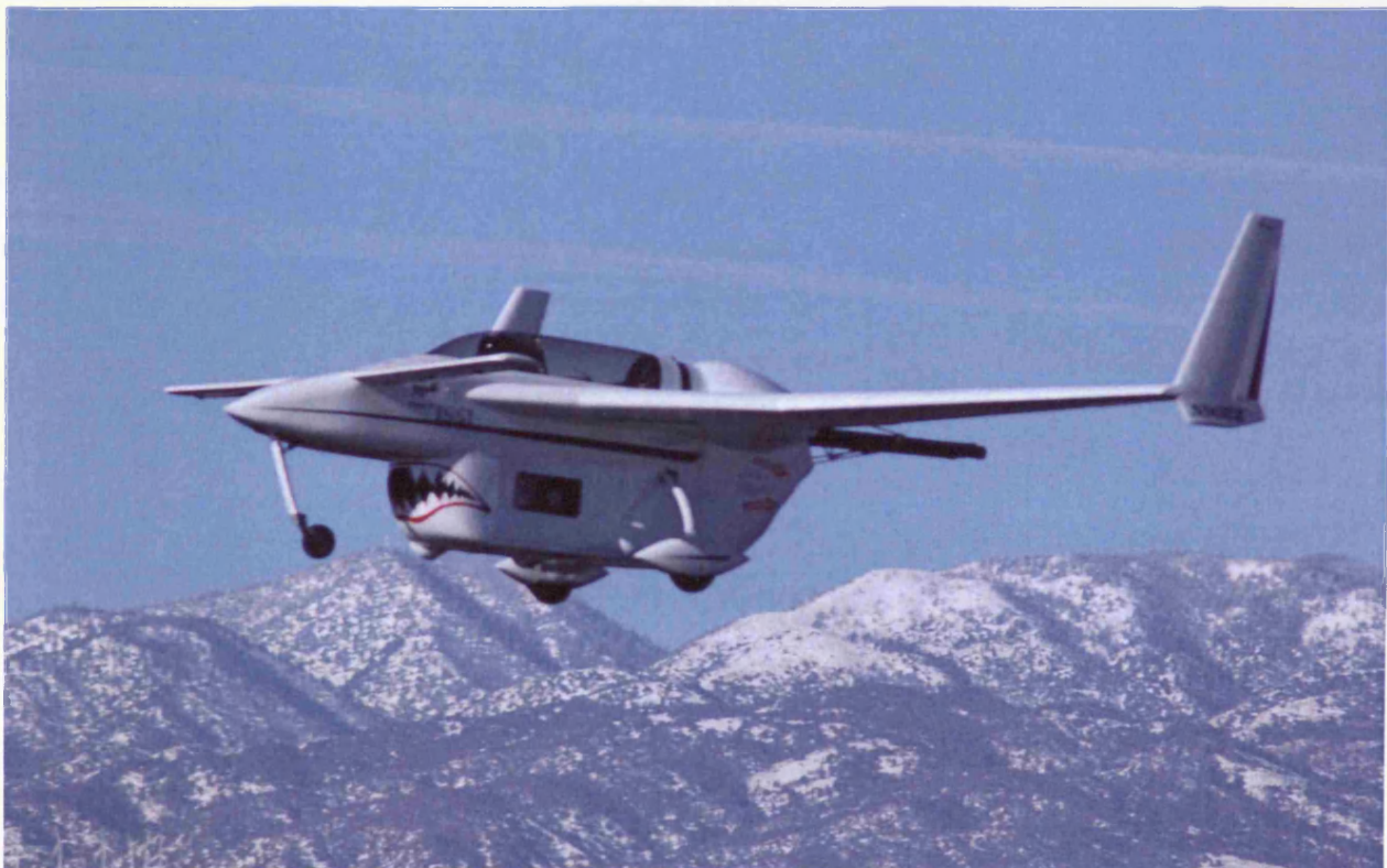
Figure 1.4: AFRL's PDE Powered Long-EZ Aircraft over the Mohave Desert [11]
