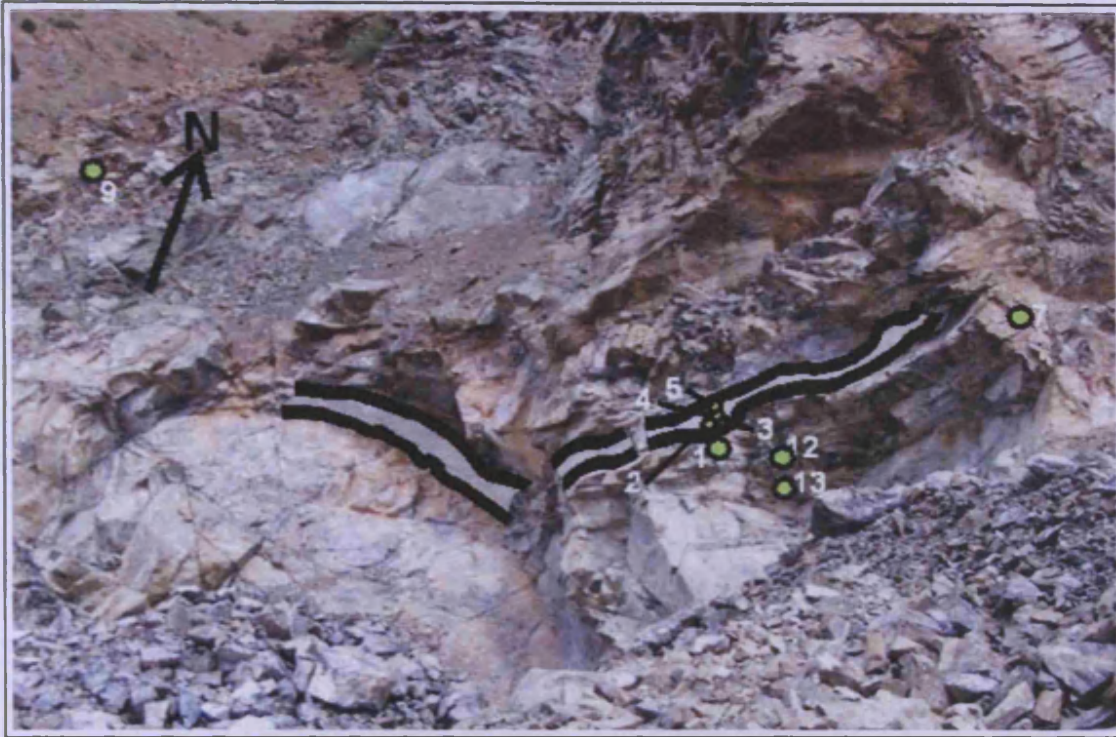
Figure 5.2: The Dereagzi outcrop, showing the remaining chromitite seam (shaded in grey) and the positions of the in-situ samples which collected. The original chromitite outcrop was much larger but has since been mined out.
