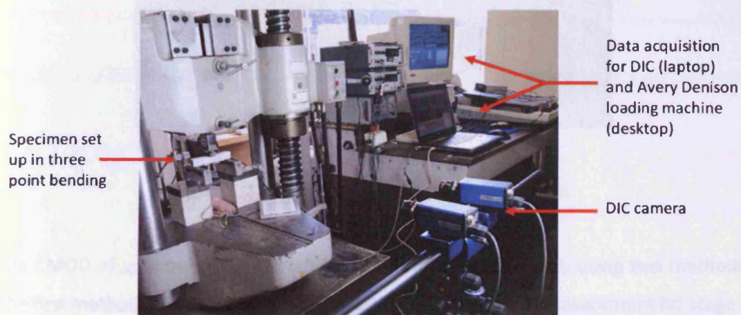
Figure 5.1 Test set up of a typical specimen subject to three-point bending with DIC measurement
