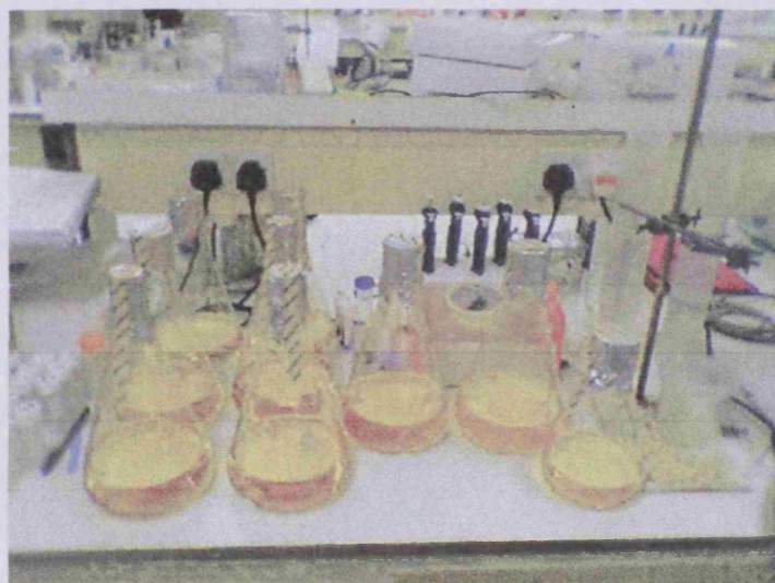
Figure 3.10. 750 ml cultures in 2 L flasks were used at 280 rpm in expression flasks. A lot of different expression conditions were tested in order to achieve the optimal expression conditions and establish an expression protocol.
