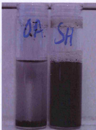
Figure 4.10: Aqueous dispersion of magnetite nanoparticles following the exchange of oleic acid (OA) surface groups with 11-mercaptoundecanoic acid (SH). Both samples have been washed extensively with water.
