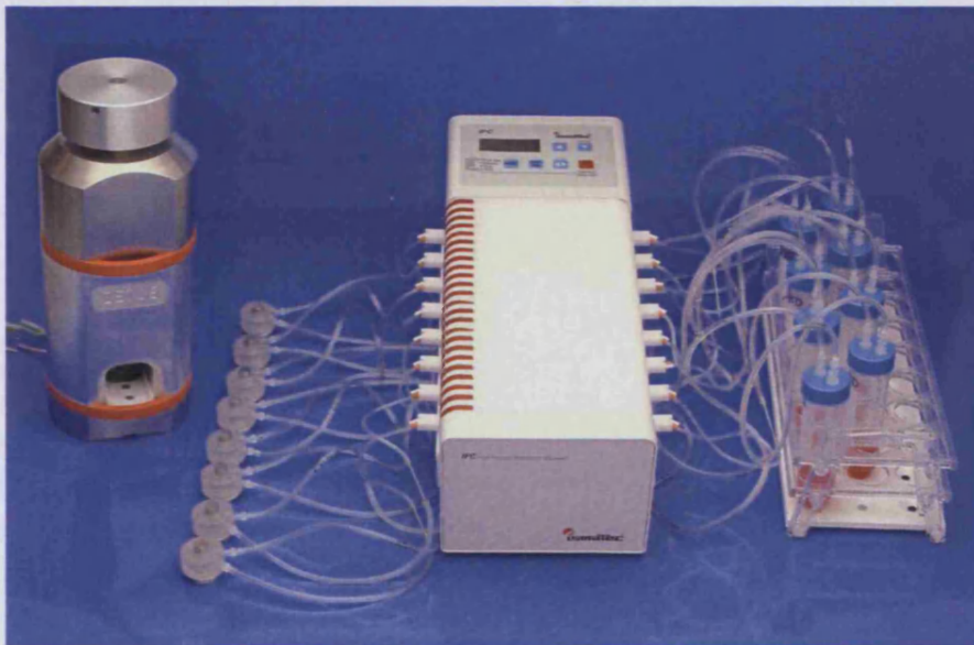
Figure 1.b.1. The Zetos culture system which comprises of a loading device, and a set of culture chambers, each with their own media supply fed from a reservoir through Tygon tubing with the aid of an Ismatech pump.
