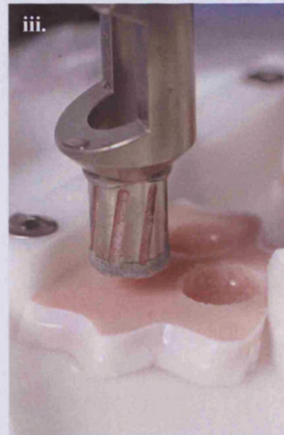
Figure 1.b.8. i.) Soft tissue removal from ovine femur under sterile conditions in a laminar flow hood. ii.) Bone slabs cut from bovine metacarpal with the Exakt band saw. iii) Cores bored from bovine metacarpal with a hollow diamond rimmed drill bit. iv) Bone cores cut parallel with an annular saw to provide surface parallelism to the cylinders. During all cutting procedures 0.9% NaCl was used for irrigation.
