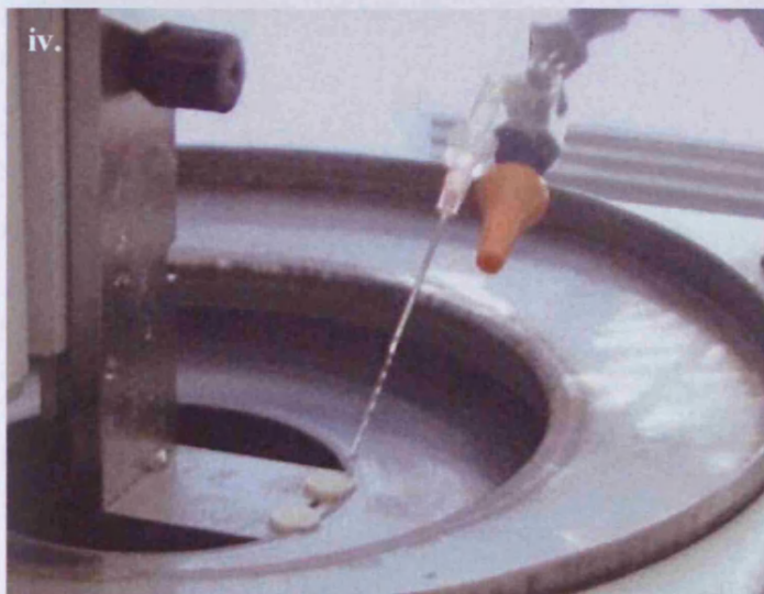
Figure 1.b.8. i.) Soft tissue removal from ovine femur under sterile conditions in a laminar flow hood. ii.) Bone slabs cut from bovine metacarpal with the Exakt band saw. iii) Cores bored from bovine metacarpal with a hollow diamond rimmed drill bit. iv) Bone cores cut parallel with an annular saw to provide surface parallelism to the cylinders. During all cutting procedures 0.9% NaCl was used for irrigation.
