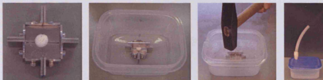
Figure 2.b.1. The novel technique to freeze-fracture bone cores. Adapted from [ap Gwyn et al., 2002]
