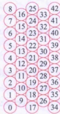
Figure 4.6: Diagram showing the indexing system used to specify individual detector pixels within the SPS.
