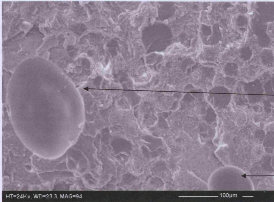
Figure 5.17: Fatigue fracture surface of 30% untreated ABS magnification x 94
