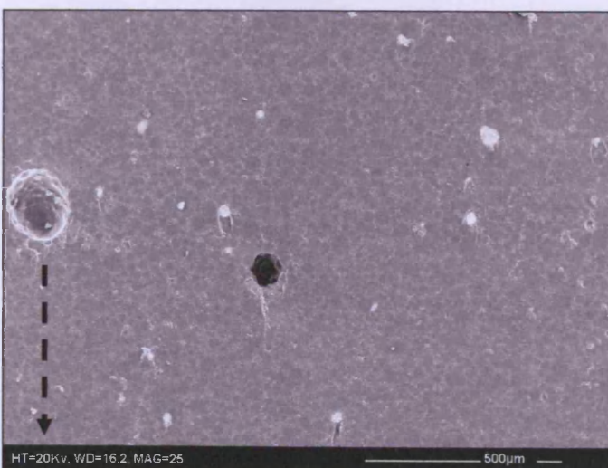
Figure 4.16: Fracture surface of 50% B866, magnification x 25
