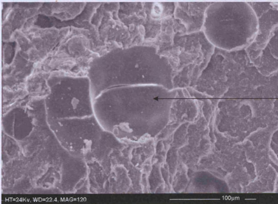
Figure 5.20: Fatigue fracture surface of 40% silane-coated ABS magnification x 120
