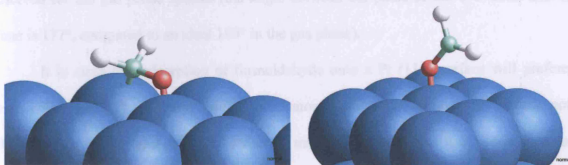
Figure 5.10: Calculated adsorption geometries for formaldehyde on a Pt (111) surface; \mu_2(\text{C},\text{O}) (left) and \eta^1(\text{O}) (right)
