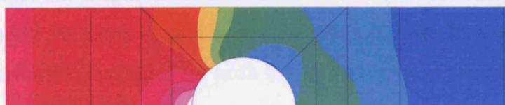
Figure 4.18: Pressure contours of the flow past a solid sphere calculated with  $K = 12$  and  $N = 8$  for  $Re = 50$ .
