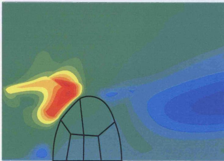
Figure 6.15: Deformed droplet with  $We = 3$  at  $t = 0.3$  and the radial velocity contours.
