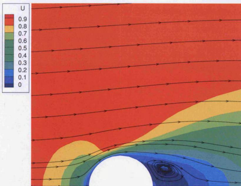
Figure 4.24: Particle tracks (streamlines) with axial velocity contours of the ambient flow over a solid sphere at  $Re = 180$ .
