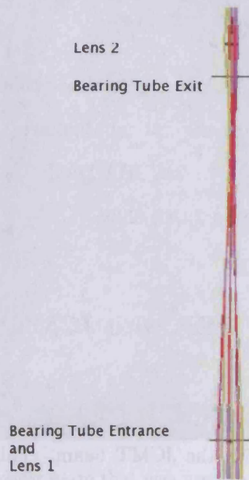
Figure 4.3: Detail of the optical setup at the JCMT. Shown is the entrance and the exit of the bearing tube and both the lenses. The length of the bearing tube is 182.5 cm. Lens 2 is 16.5 cm from the exit of the bearing tube.
