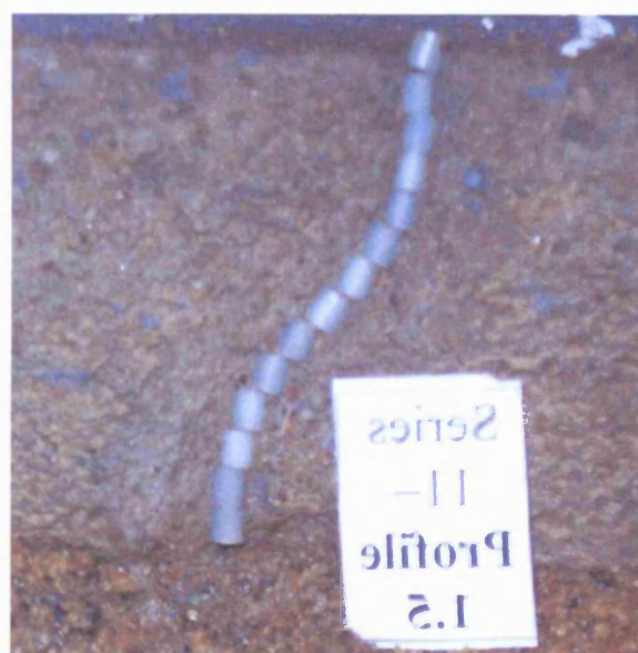
Figure 5.5.22. Example of the conversion of subsurface marker profiles into numeric data.
