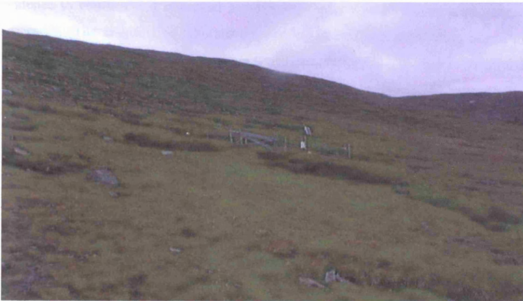
Figure 8.0.1. The fully constructed field-monitoring station. (Photograph: Charles Harris). Note: the turf-banked solifluction lobes with risers of 0.5 – 1.25 m.
