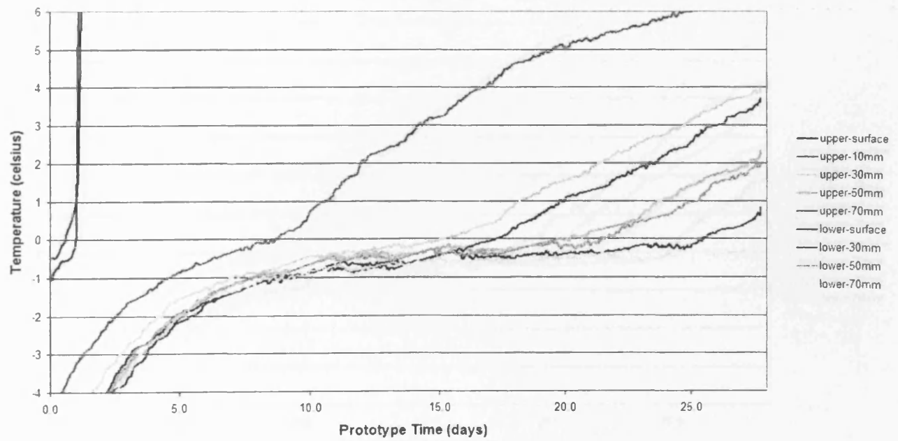
Figure A.5. Thermal data recorded during the third thaw phase of series 4D/NS.
