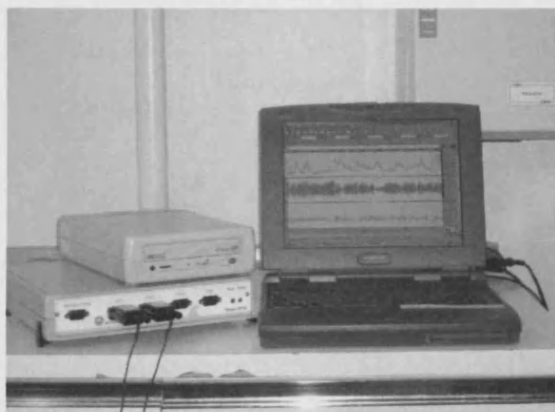
Fig. 5.2. The physiological amplifier (Biopac MP30) and laptop PC (Toshiba pro 4200 series).
