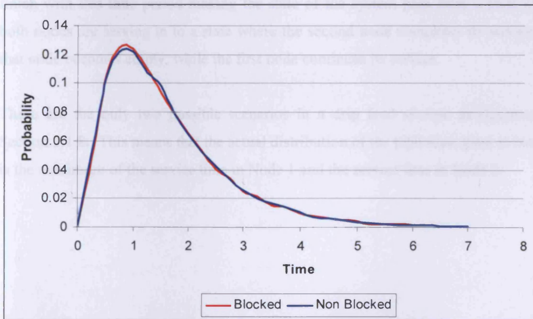
Figure 3.17 - Time spent in Node 1 of a drip feed system for blocked and non blocked customers, with service rates equal to 1.
