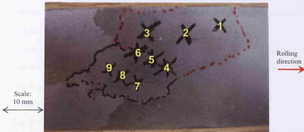
Figure 6.42. Photo of the uncoated grain-oriented 3%SiFe electrical steel sample. The numbers indicate the location where the ferrite sensor was placed for measurement of Barkhausen noise (1 is P1 in figures, etc)
