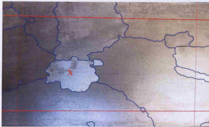
Figure 6.67. Picture of the area scanned on the grain-oriented 3%SiFe electrical steel sample (red lines indicate the area scanned, and the blue lines outline the grains)
