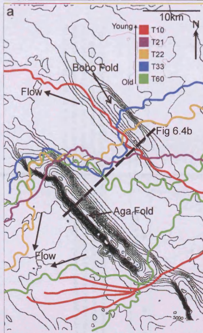
Figure 6.4: The contour map shown in a shows the time structure at the base of the growth sequence (T60 horizon in b) for the Niger Delta study area. Coloured lines represent the paths of several submarine channel systems located at various stratigraphic levels within the growth sequence, as shown in the seismic profile in b. This figure shows that, from the onset of growth of the Aga fold, submarine channel systems were diverted around the lateral tip regions of the fold with the location of the diversions remaining fairly constant – ie lateral propagation of the fold along strike was not a significant factor in controlling the pathways of submarine channel systems during growth of the Aga fold. Compare with the example of fold growth documented in chapter 5.
