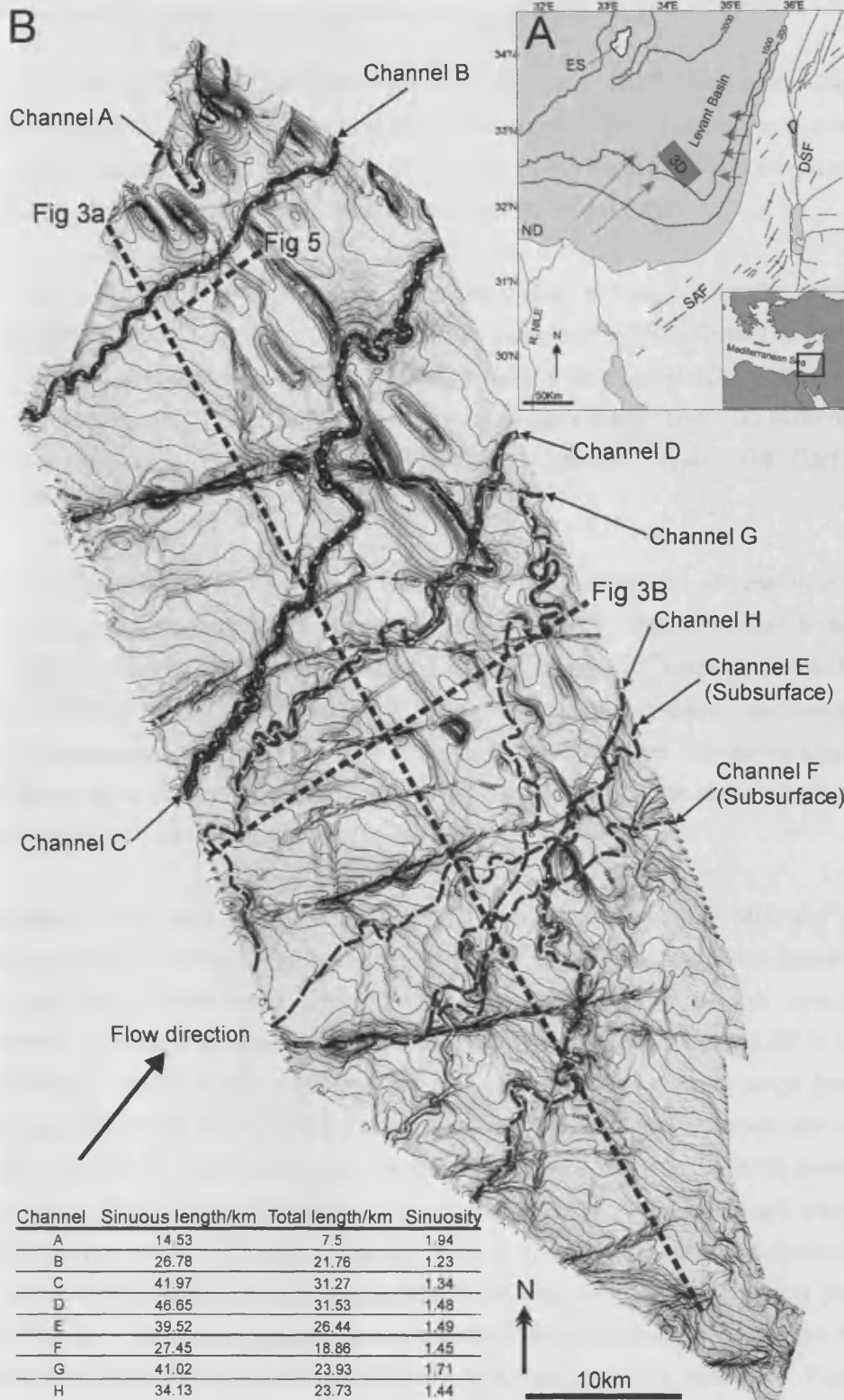
Figure 3.1: 3.1a shows a location map of the 3D seismic survey used in this study. DSF = Dead Sea Fault System, SAF = Syrian Arc Fold Belt, ES = Eratosthenes Seamount, ND = Nile Delta. Arrows indicate direction of salt flow from the Nile Delta and Levant Margin. Adapted from Vidal et al. 2000, with salt movement direction from Netzeband et al. 2006. 3.1b shows a dip attribute map of the seabed over the 3D survey area. This map is draped with time contours (Interval = 10ms TWT). The map shows channel levee systems A, B and C which are described in this study. Several other channel levee systems are present and some key characteristics of these are summarised in the inset table.
