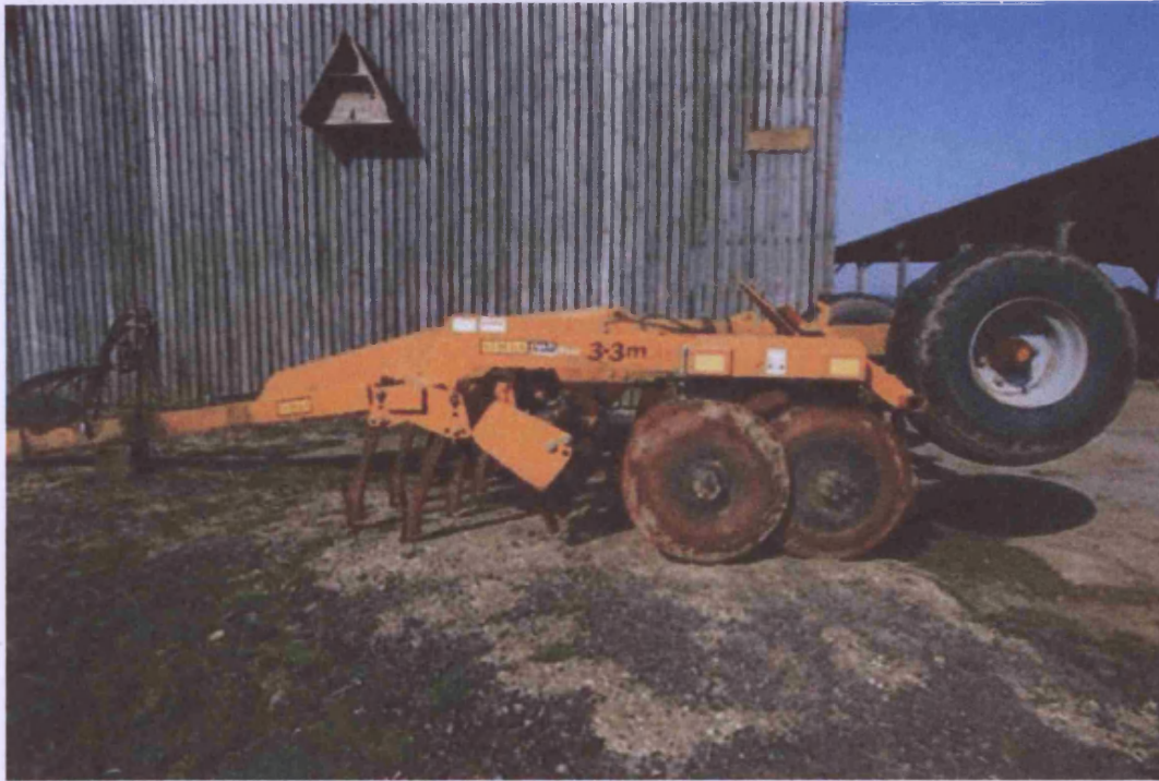
Fig. 4.3. Soil for the minimum tillage treatment was prepared using the 3.3 m Simba Cultipress (pictured).
