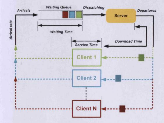
Figure 5.1: Local rendering system architecture and parameters for single server queuing.
