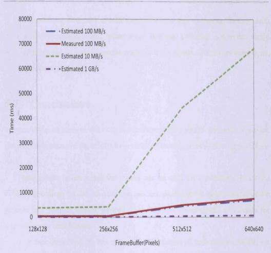
Figure 5.14: Local rendering for different networks bandwidths.
