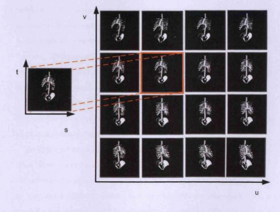
Figure 2.3: 4D Light Field representation in terms of an array of images taken at different positions in the (u, v) plane.
