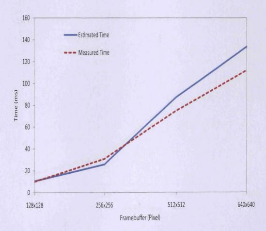
Figure 5.6: On-demand rendering: model and experimental timing results for one visualization client and a random navigation model.
