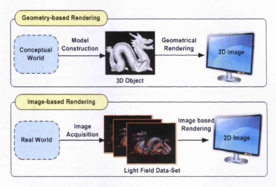
Figure 1.1: Geometry-based versus Image-based Rendering.
