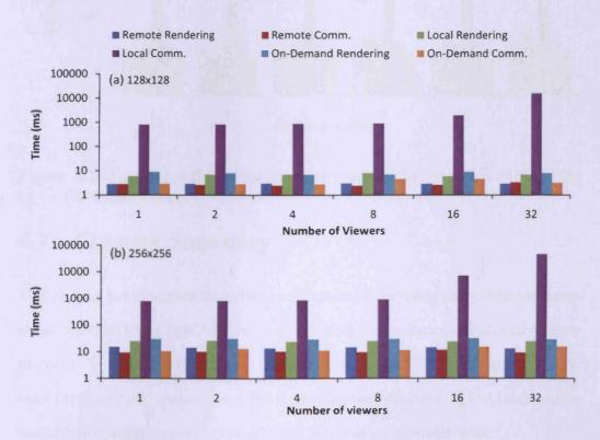
Figure 4.6: Time for different numbers of viewers for (a)  $128 \times 128$  and (b)  $256 \times 256$  dataset sizes.
