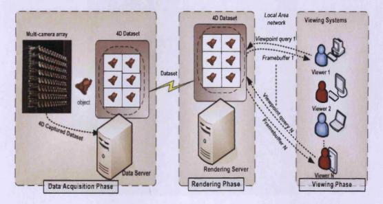
Figure 3.1: System Overview. In the Data Acquisition phase a 4D dataset is created. The Rendering phase performs interpolation across multiple images. In the Viewing phase viewpoint queries are sent and the received output frame buffers are loaded for display.
