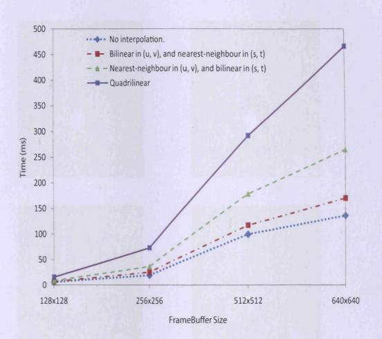
Figure 4.2: The rendering time for different interpolation schemes.
