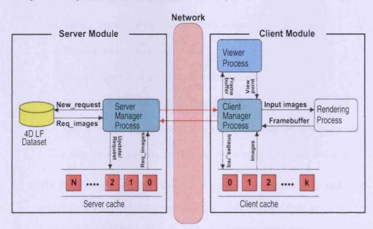
Figure 3.5: The architecture of an on-demand transmission model.
