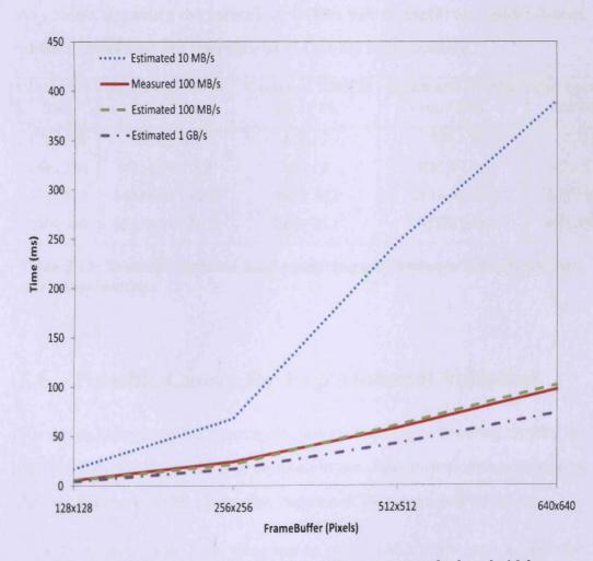
Figure 5.13: Remote rendering for different networks bandwidths.
